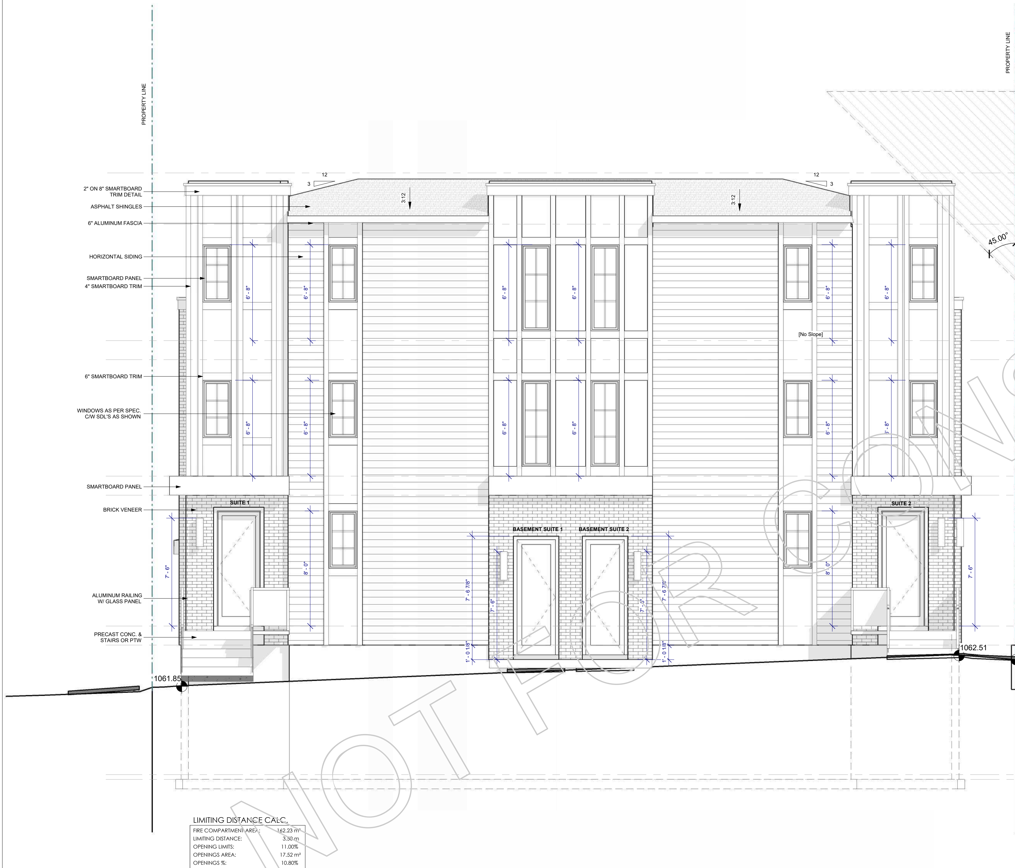
1 BLDG B - FRONT ELEVATION 1/4" = 1'-0"
