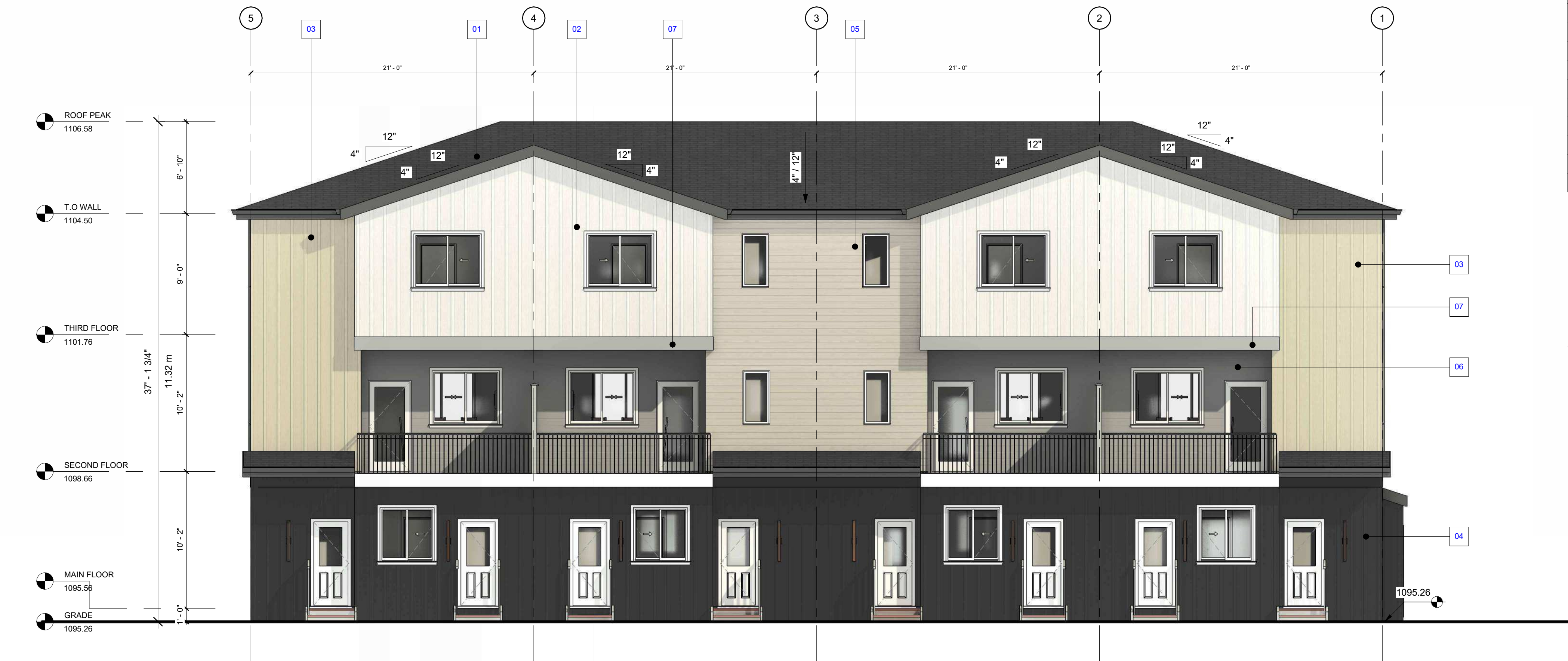
1 BUILDING 6 - WEST ELEVATION A3.1(6) 3/16" = 1'-0"
