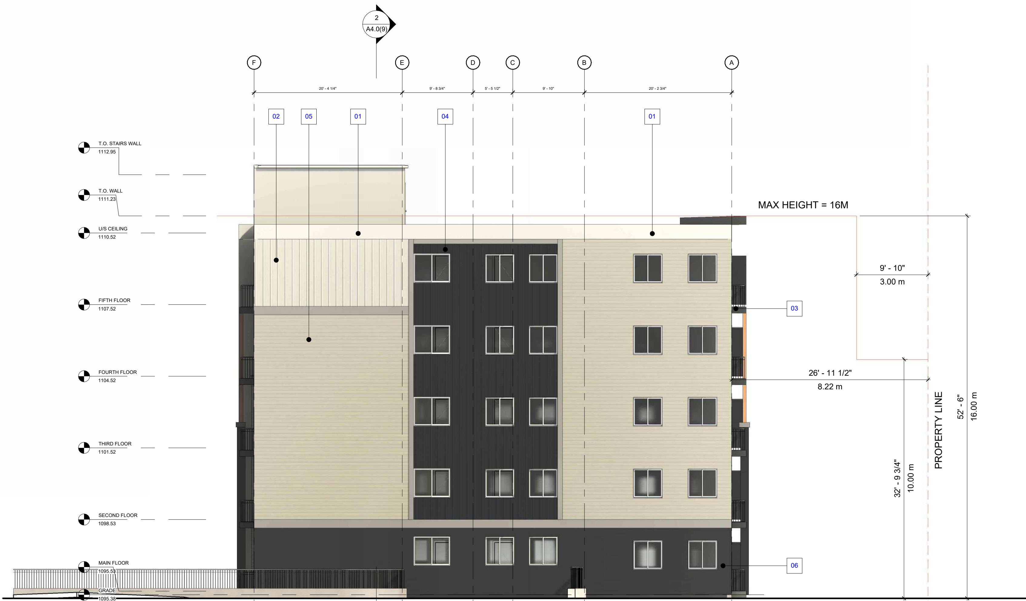
1 BUILDING 9- NORTH ELEVATION A3.1 (9) 1/8" = 1'-0"
