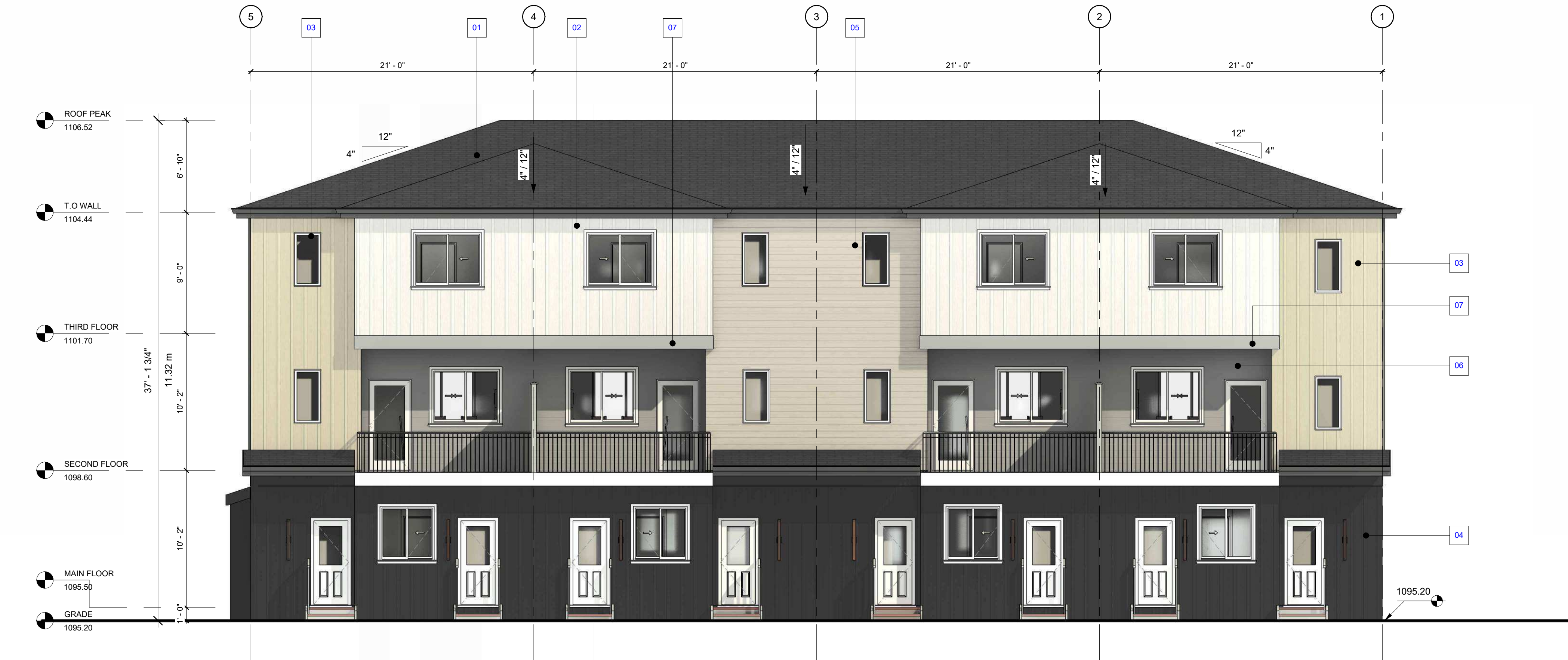
1 BUILDING 2 - NORTH ELEVATION A3.1(2) 3/16" = 1'-0"
