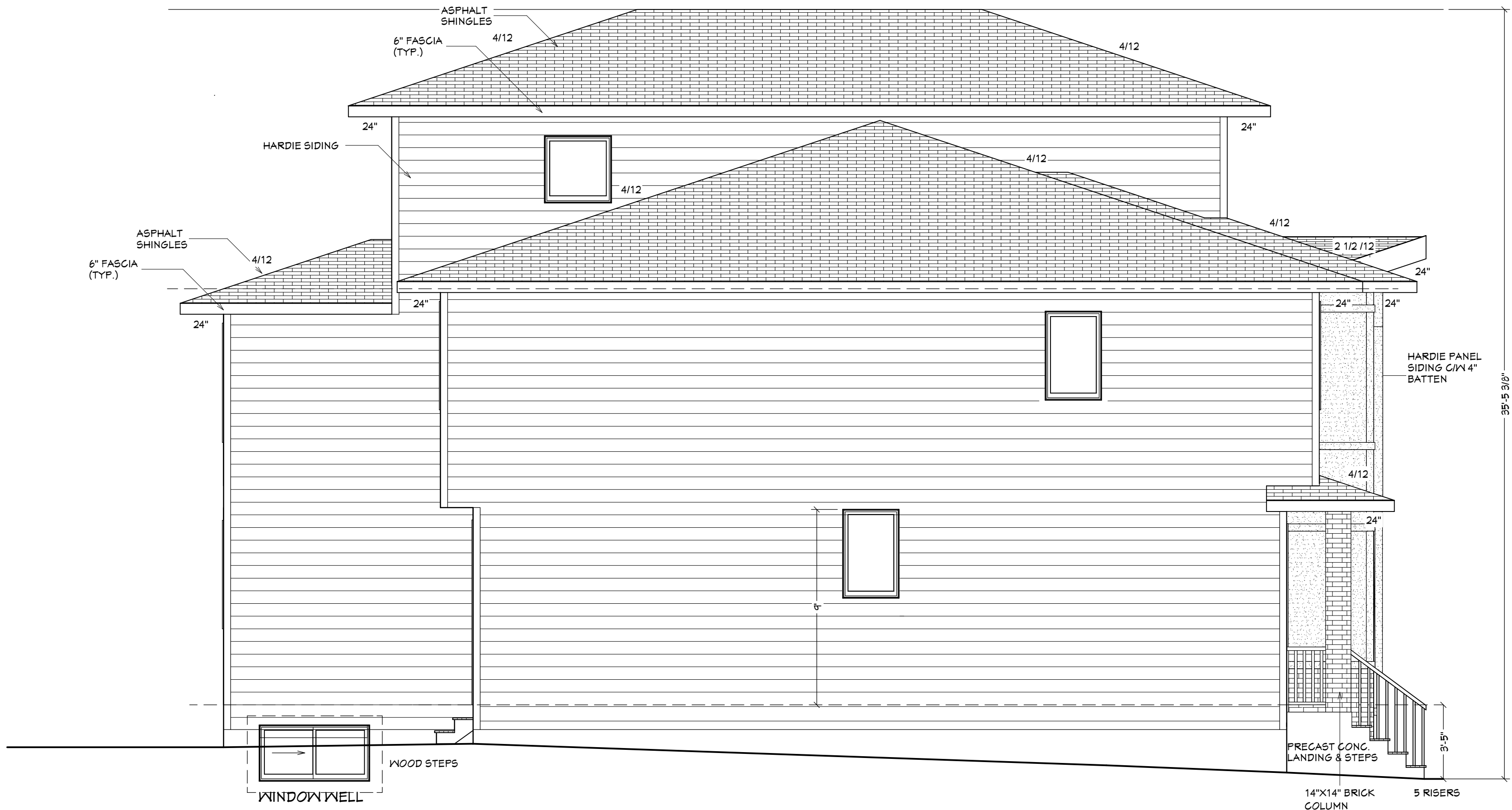
NORTH WEST ELEVATION
