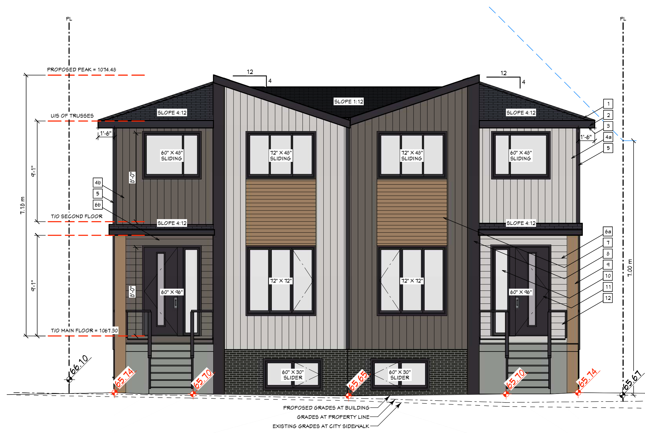
FRONT ELEVATION (EAST) SCALE: 3/16" = 1'-0"
