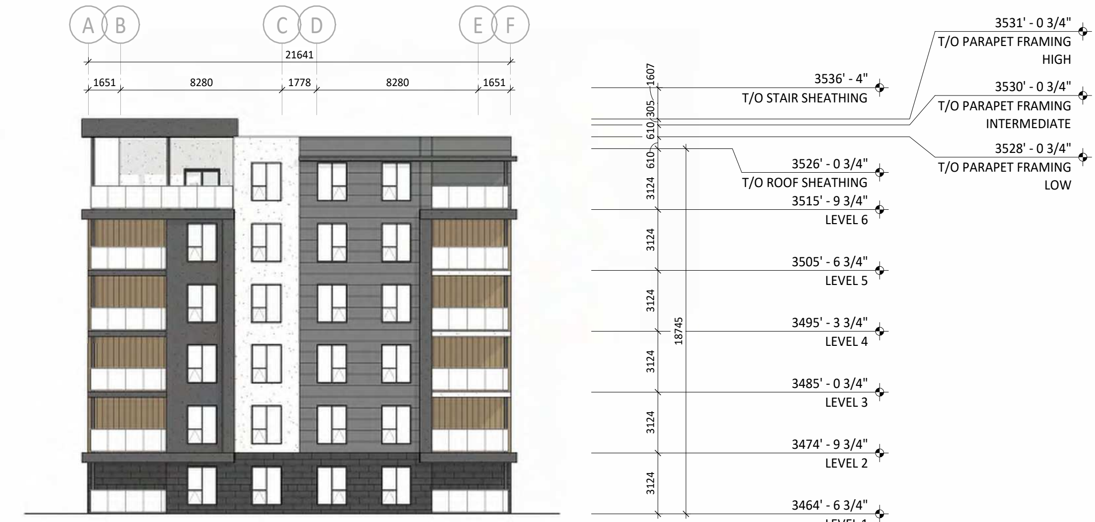
4 BLDG 2 - WEST ELEVATION DP40.01 1/16" = 1'-0"
