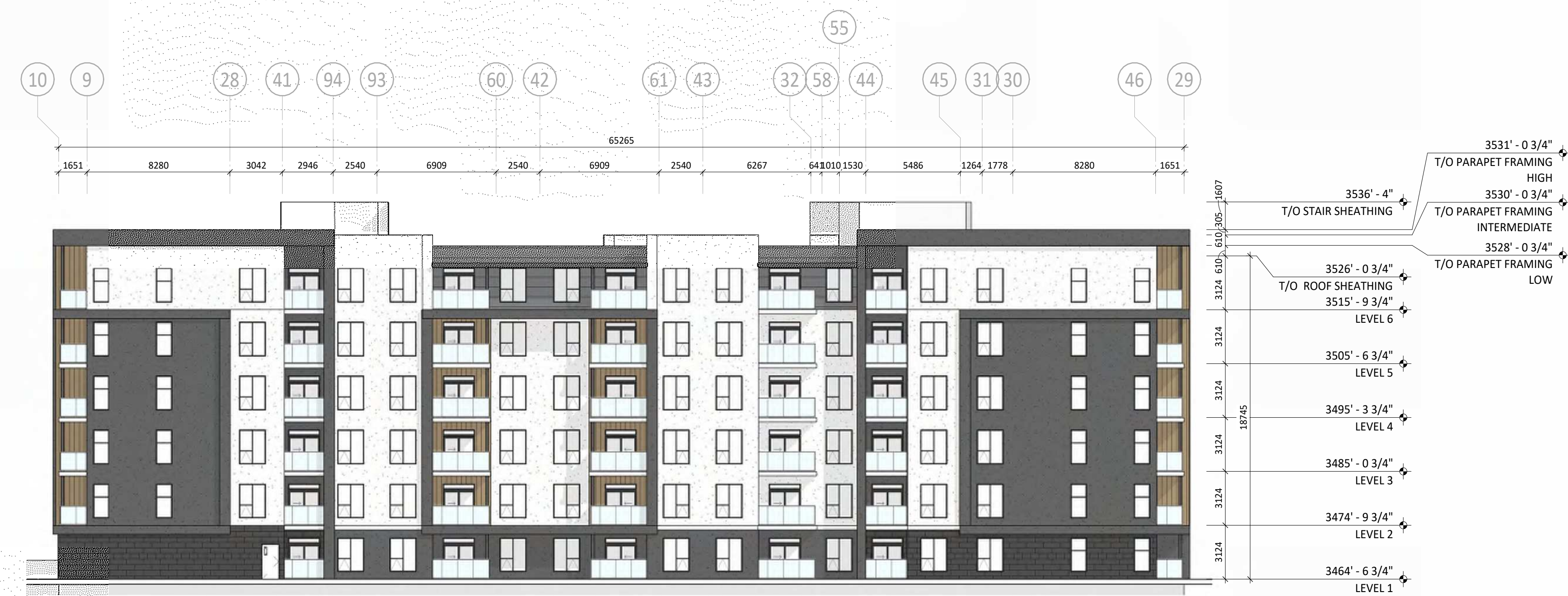
2 BLDG 3- NORTH ELEVATION DP40.01 1/16" = 1'-0"
