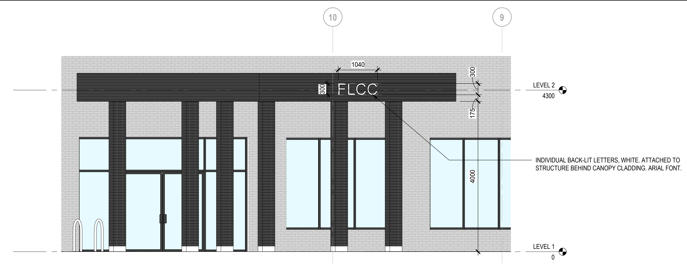
3 BUILDING SIGNAGE ELEVATION A-201 SCALE: 1:50
