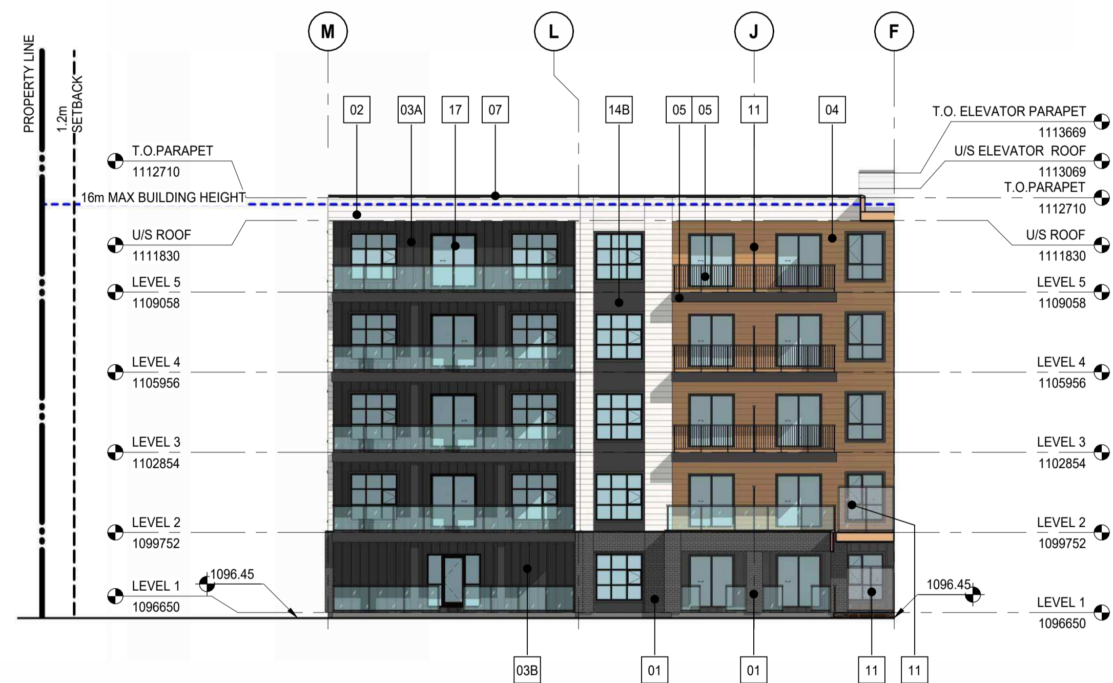
3 COURTYARD ELEVATION LOOKING EAST DP40-03-02 SCALE: 1:150
