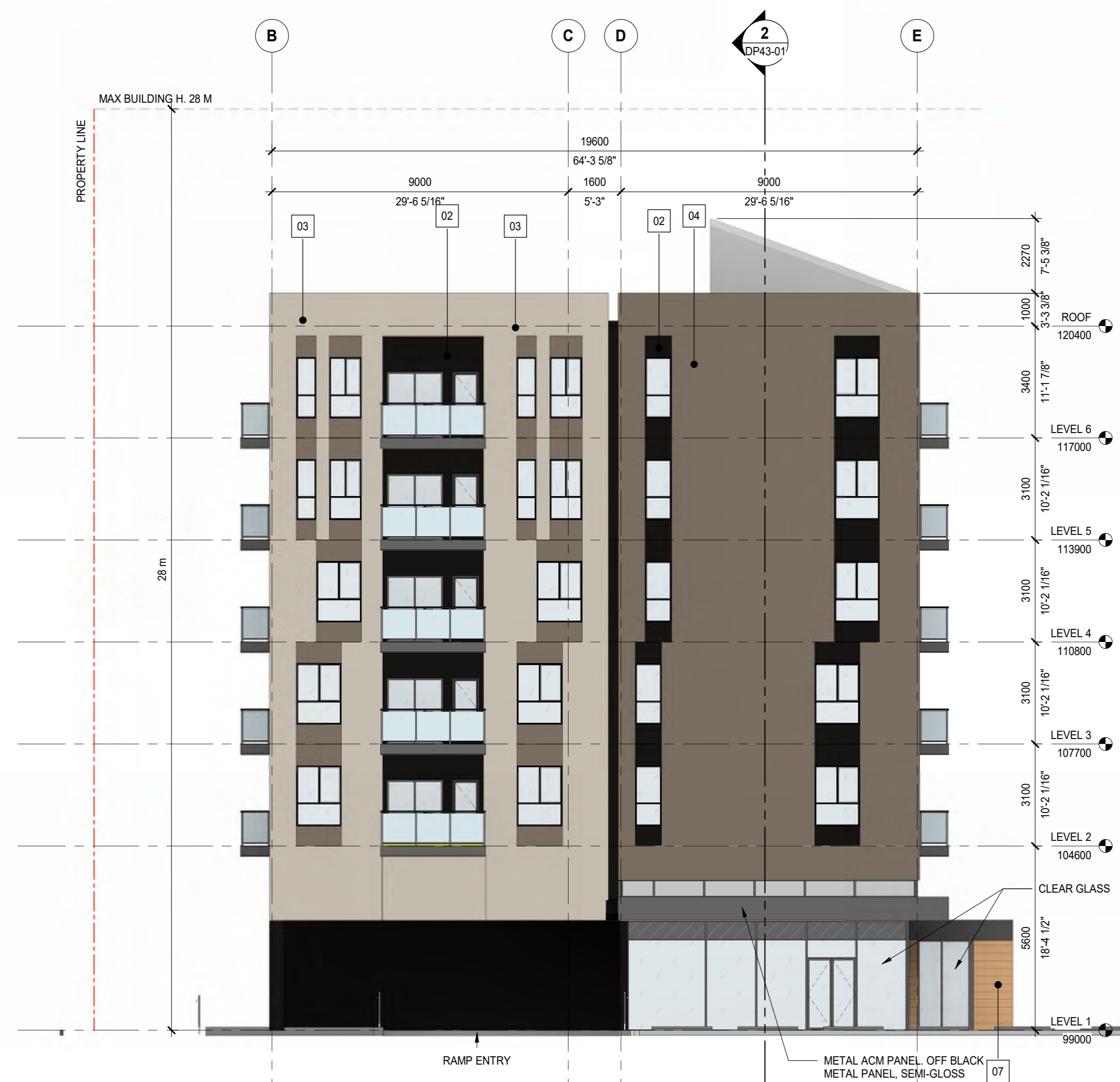
2 BUILDING 3- NORTH ELEVATION SCALE: 1:100
