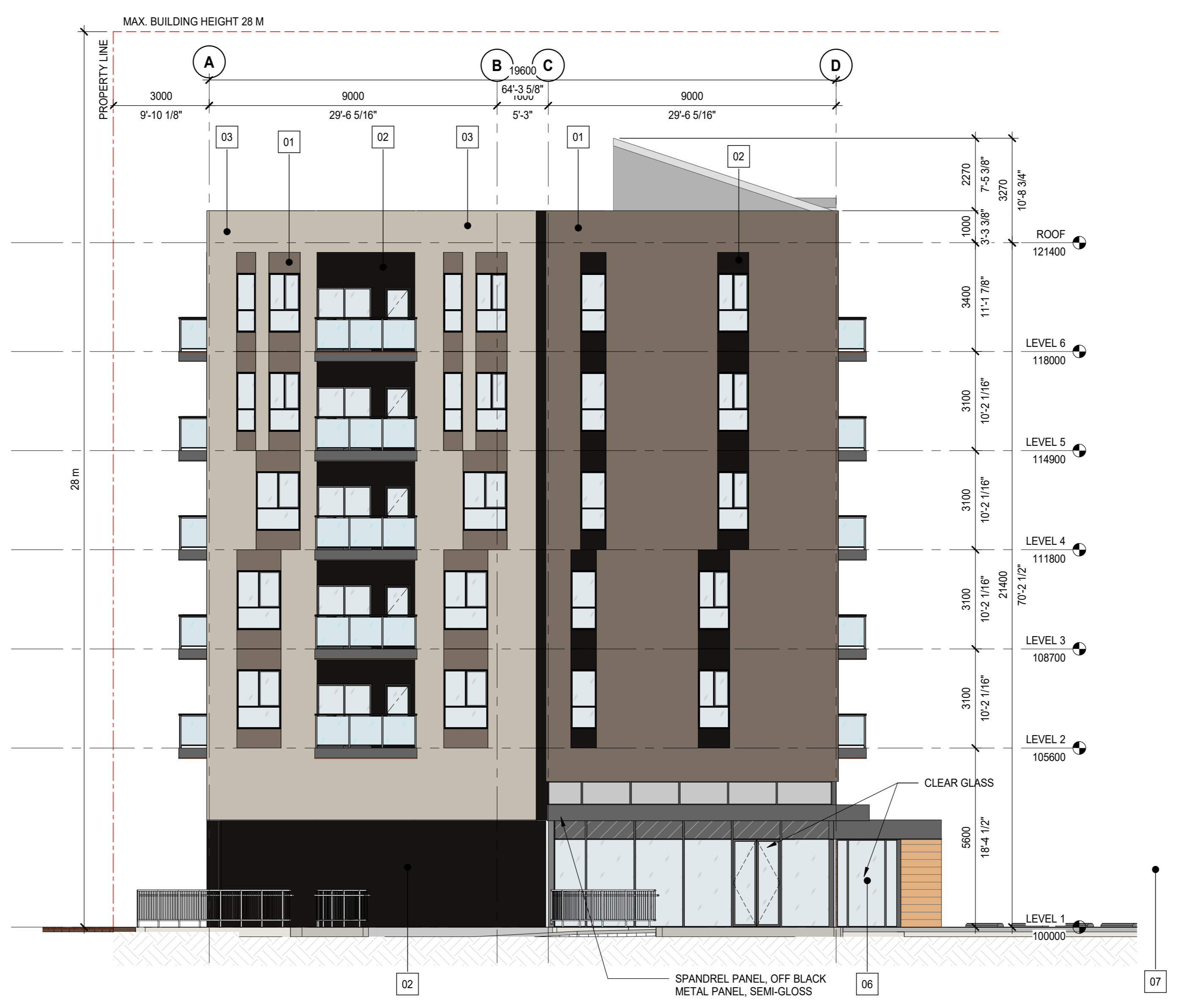
2 BUILDING 2- EAST ELEVATION SCALE: 1:100
