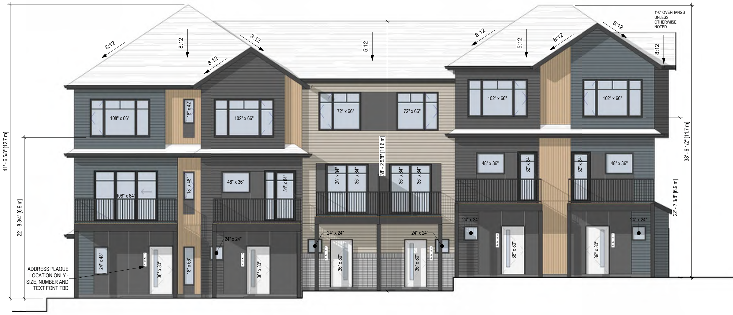
1 BLOCK 05 - NORTH WEST ELEVATION DP304 1/8" = 1'-0"
