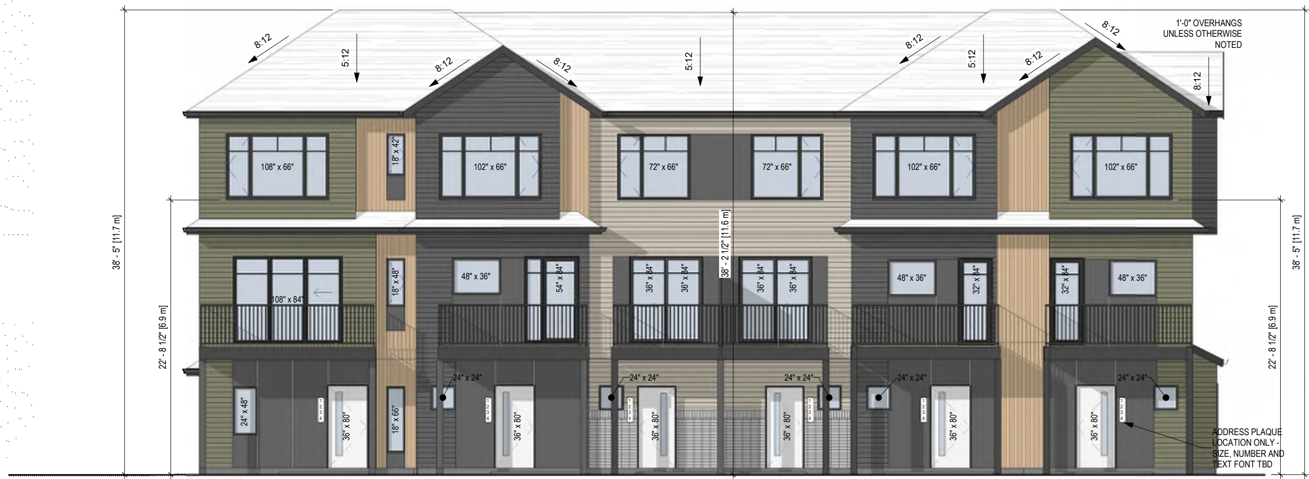
1 BLOCK 07 - SOUTH ELEVATION 1/8" = 1'-0"
