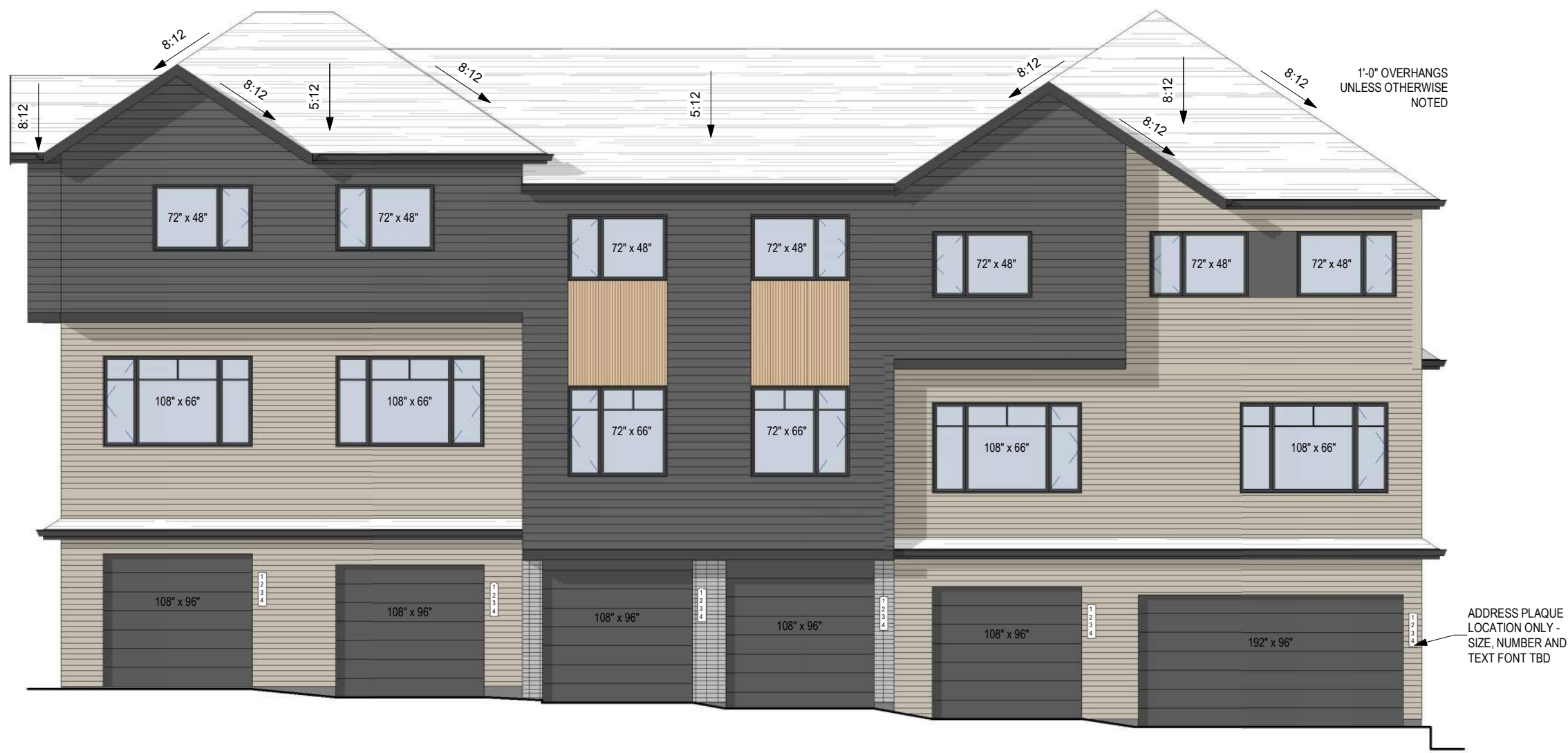
3 BLOCK 05 - SOUTH EAST ELEVATION DP304 1/8" = 1'-0"
