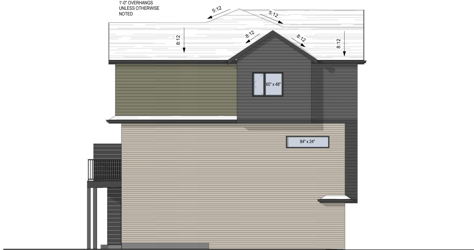
2 BLDG 07 - EAST ELEVATION DP306 1/8" = 1'-0"
