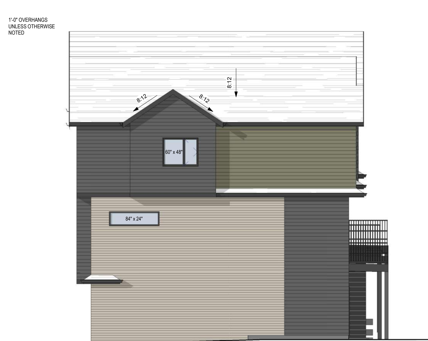
2 BLDG 09 - NORTH ELEVATION DP308 1/8" = 1'-0"
