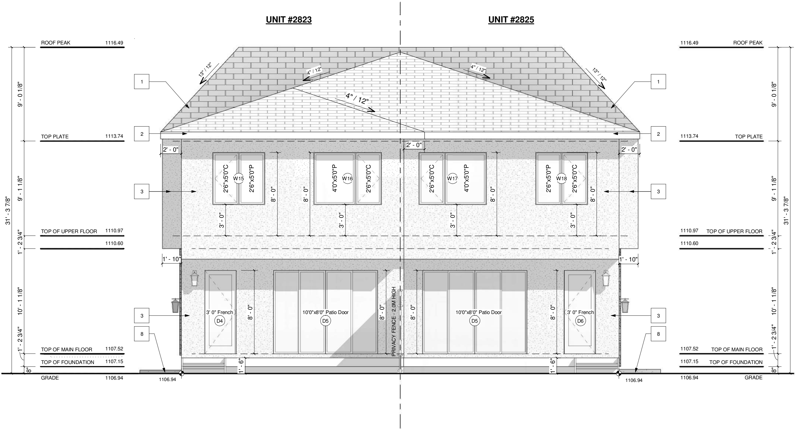
REAR ELEVATION SCALE: 3/16" = 1'-0"
