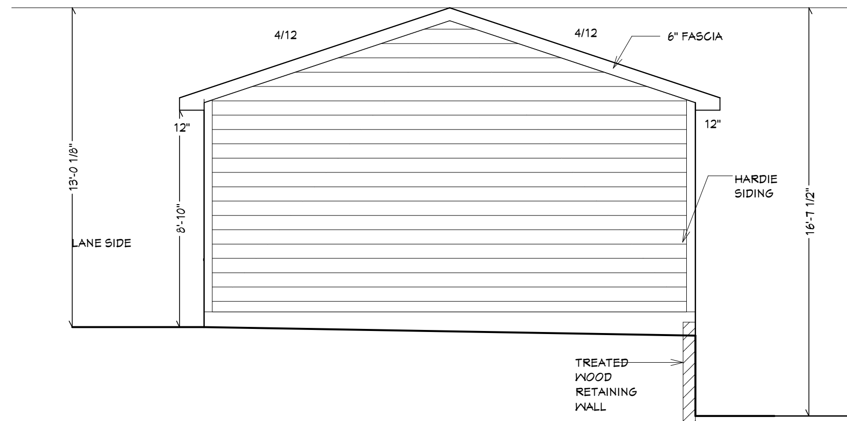
RIGHT ELEVATION (NORTH)
