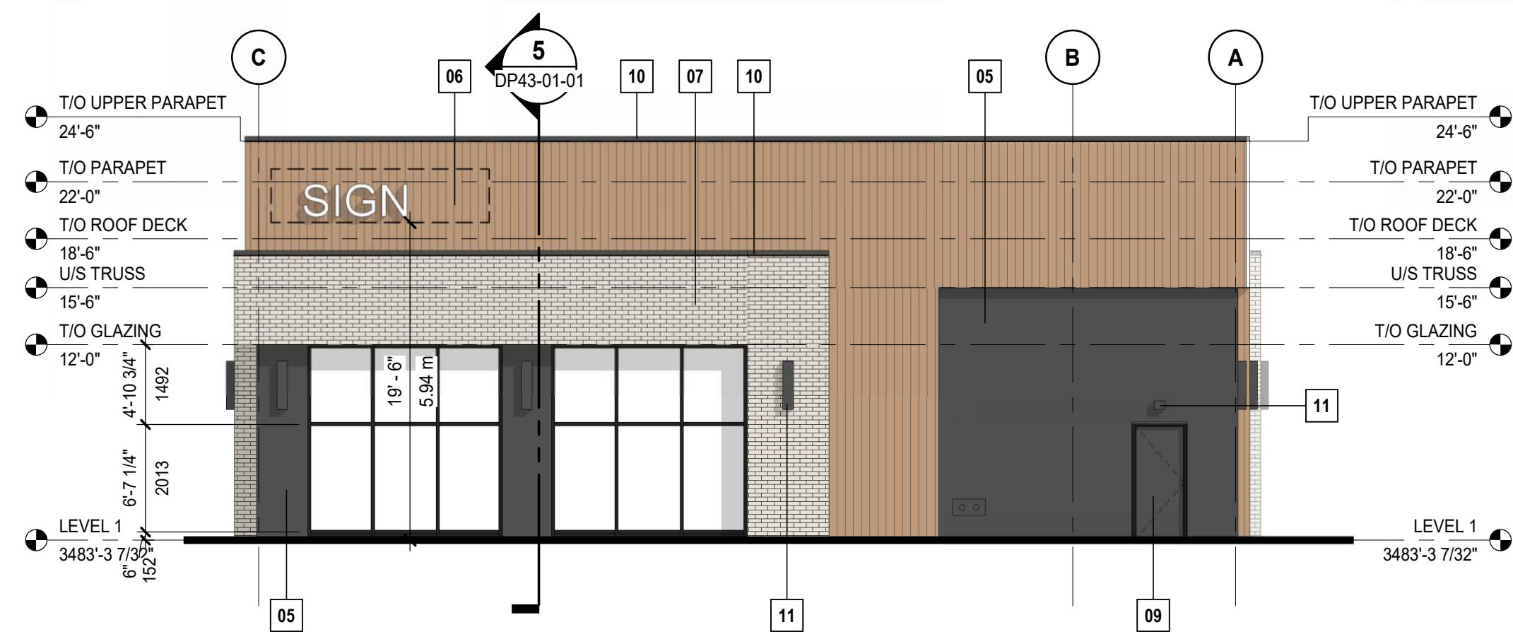
4 BUILDING 03 - OVERALL BUILDING ELEVATION - SOUTH DP40-03-01 SCALE: 1:100
