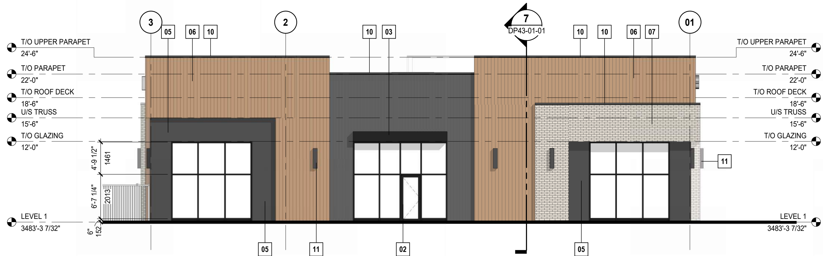
3 BUILDING 03 - OVERALL BUILDING ELEVATION - WEST DP40-03-01 SCALE: 1:100
