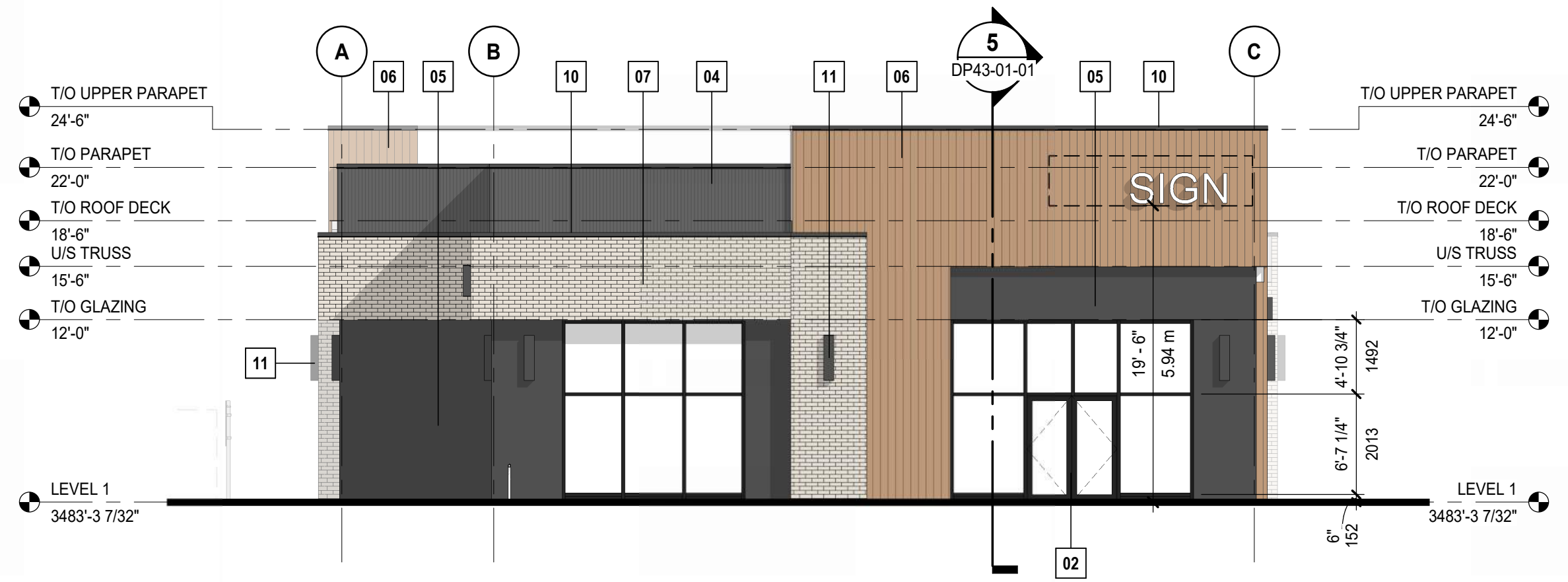
2 BUILDING 03 - OVERALL BUILDING ELEVATION - NORTH DP40-03-01 SCALE: 1 : 100
