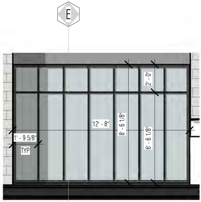
3 REAR UPPER WINDOW ELEVATION 1/4" = 1'-0"
