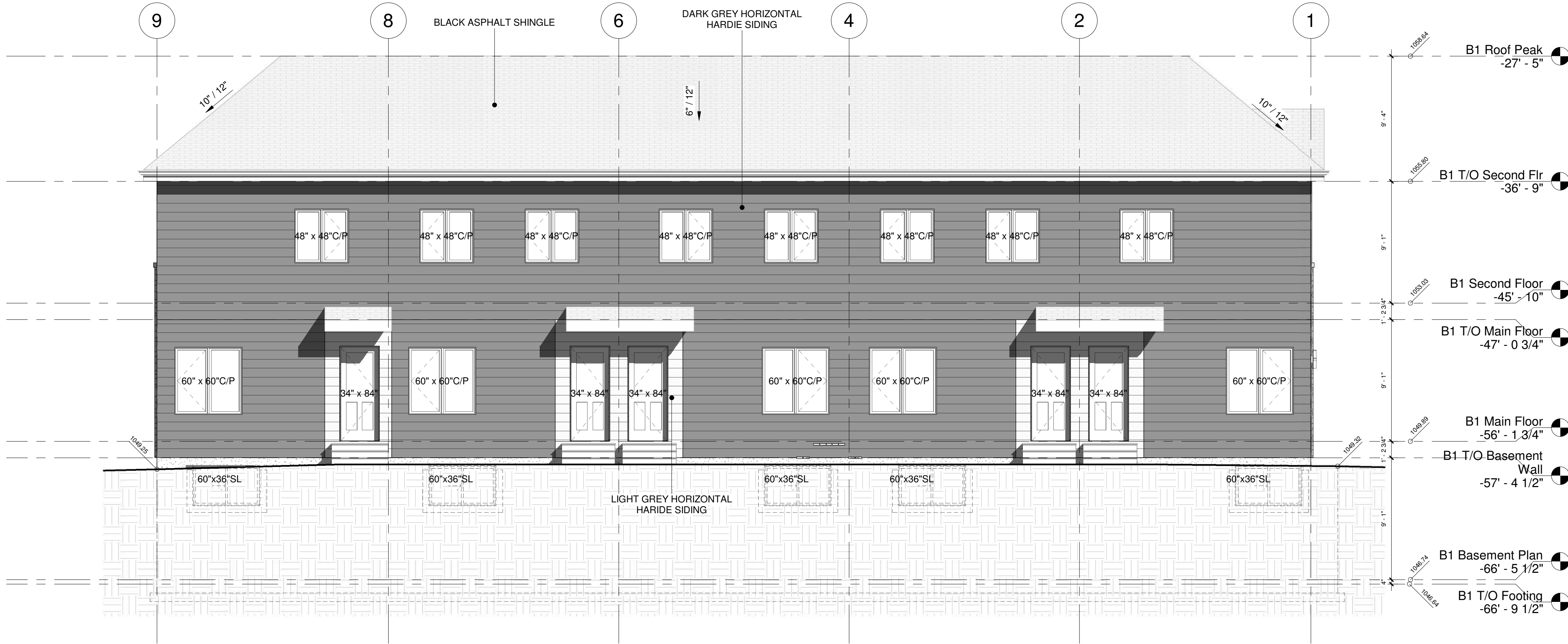
2 Building 1 South Elevation 3/16" = 1'-0"
