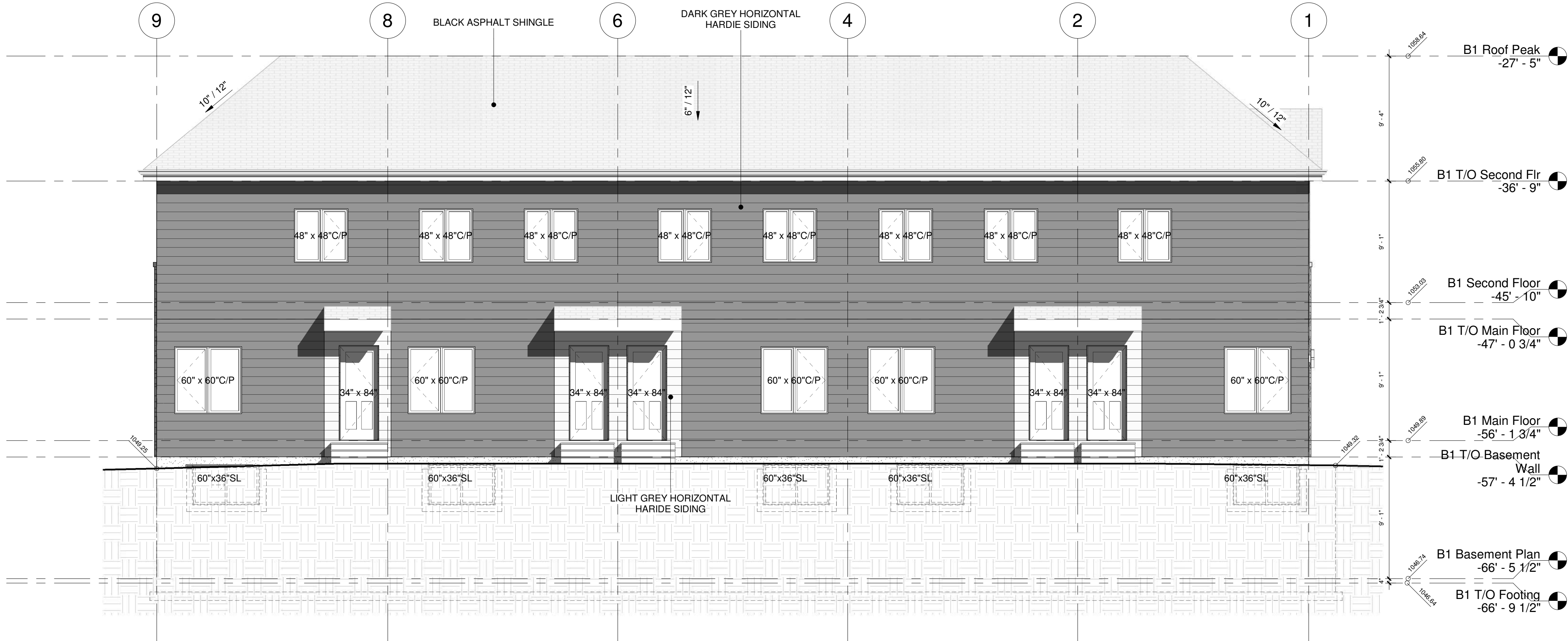
2 Building 1 South Elevation 3/16" = 1'-0"
