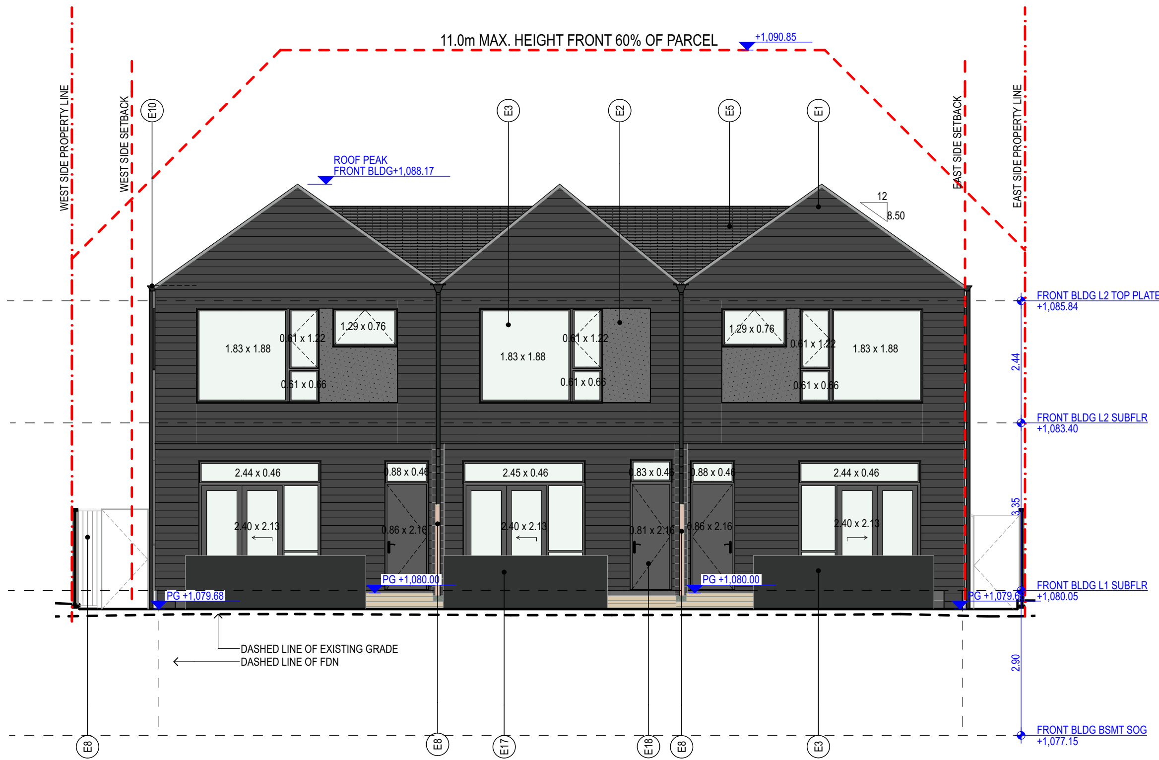
2 S1 SOUTH ELEVATION - FRONT BLDG SCALE: 1:75
