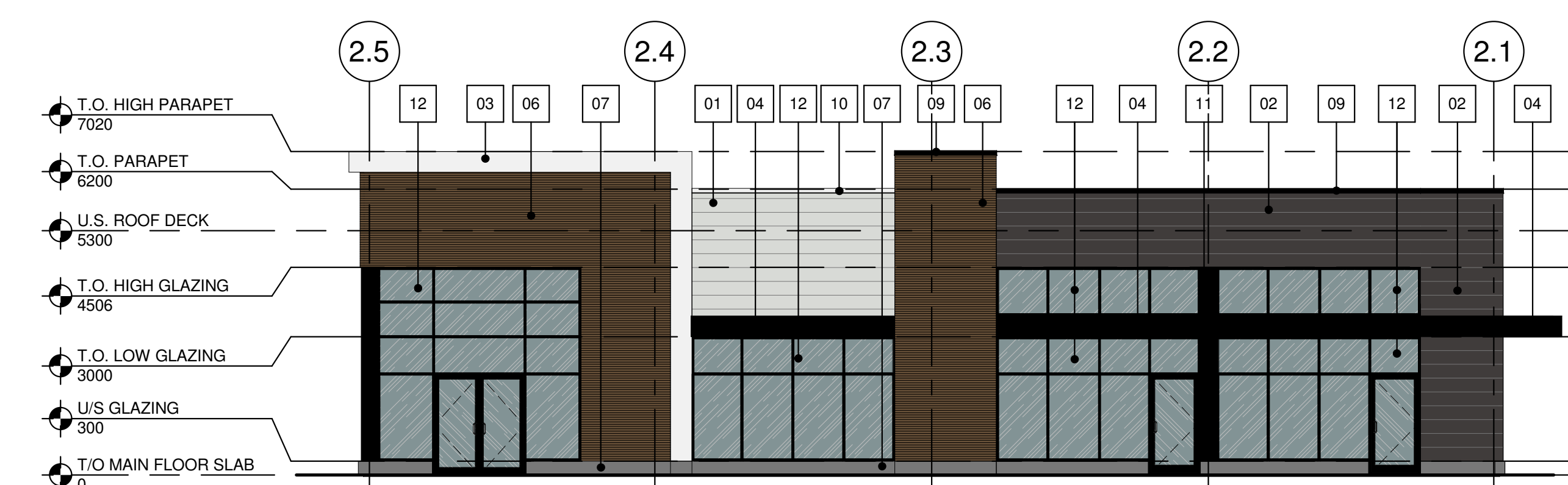
1 NORTH ELEVATION (COLOURED) 1 : 100
