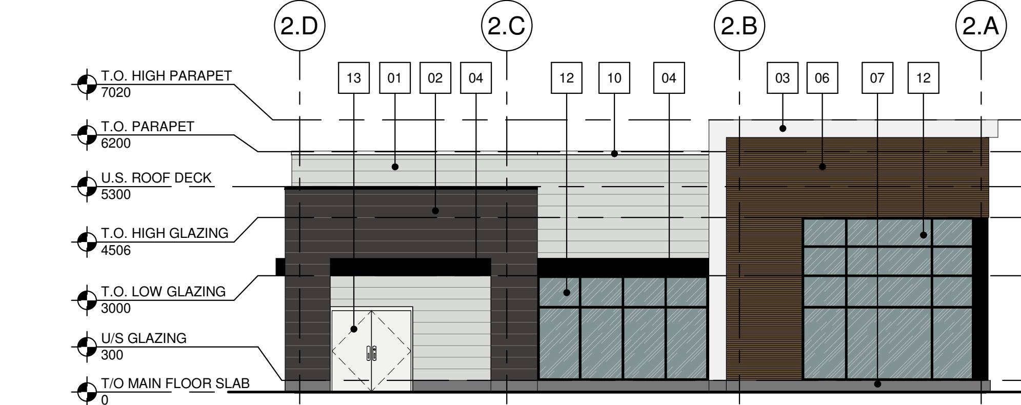
4 EAST ELEVATION (COLOURED) 1 : 100
