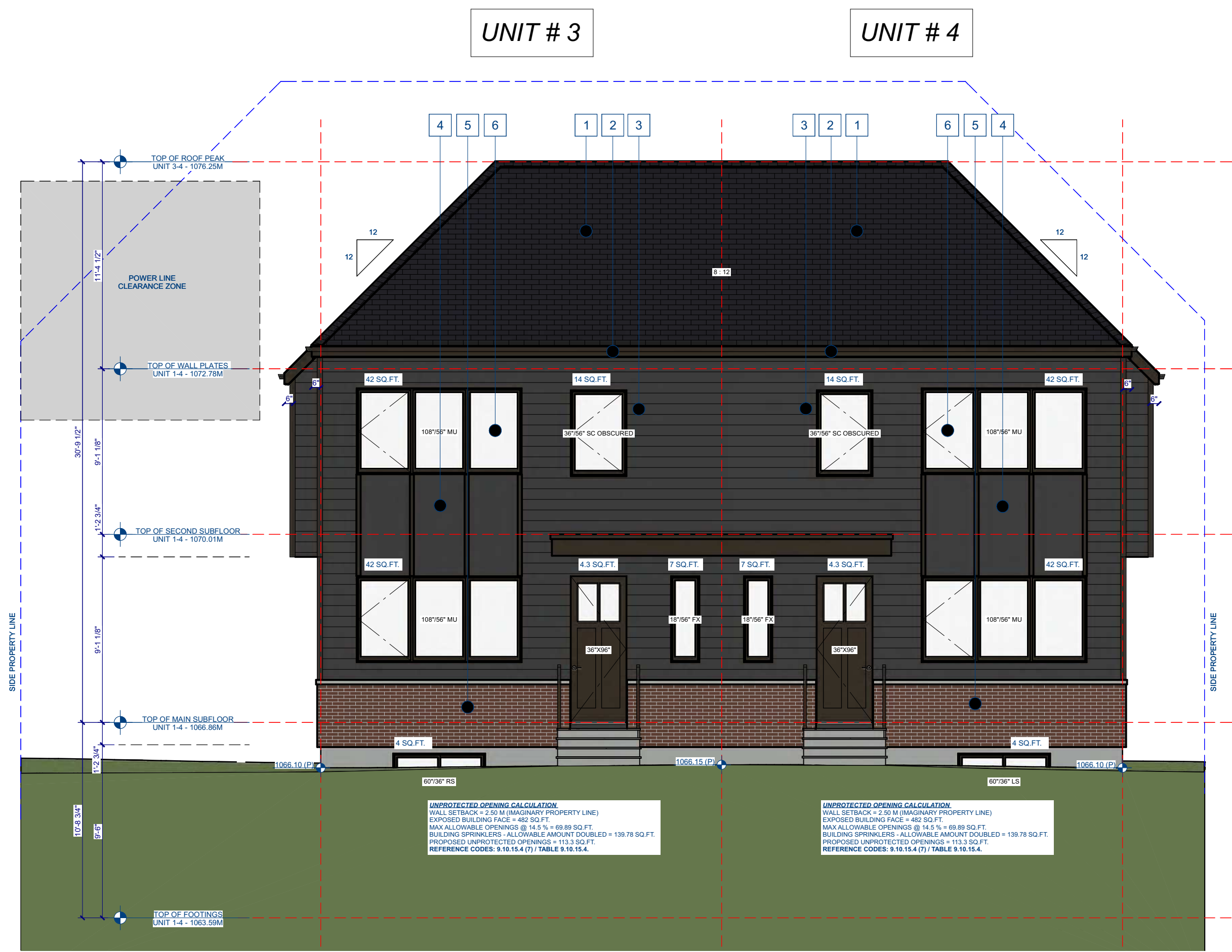
2 FRONT ELEVATION - REAR BUILDING A5 SCALE = 3/16" = 1'-0"
