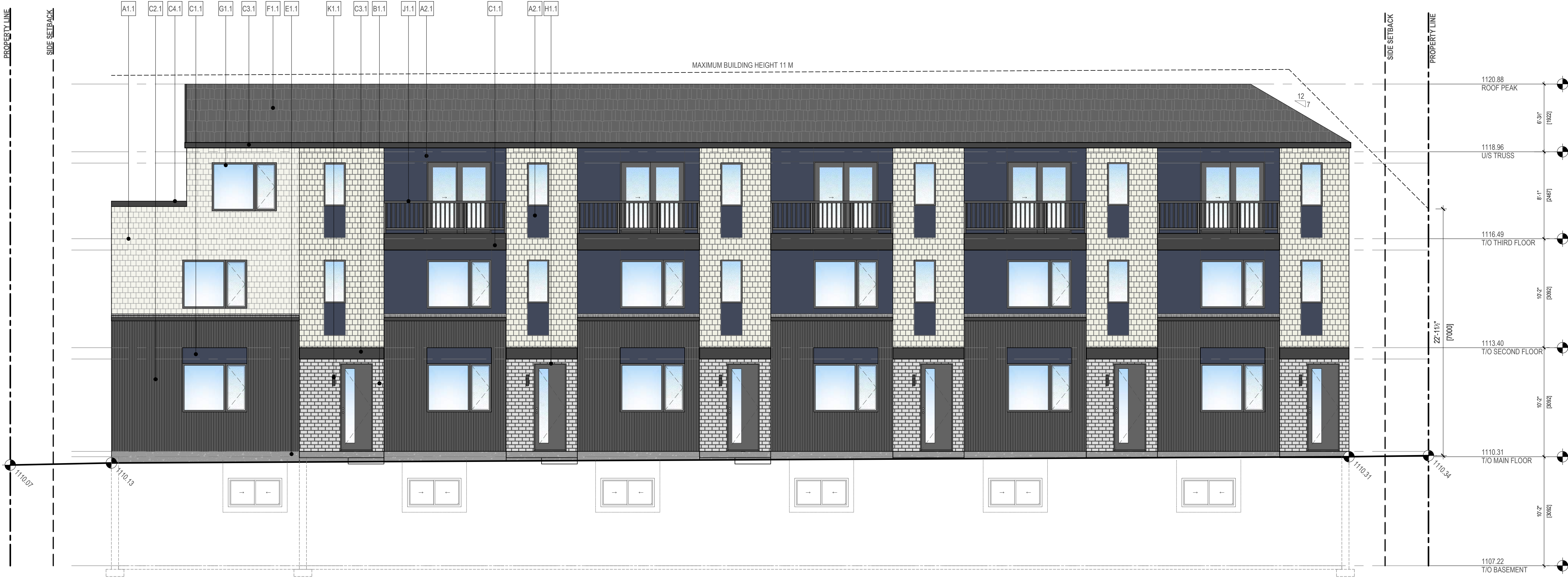
1 BUILDING A - SOUTHEAST ELEVATION DP.401 SCALE: 3/16" = 1'-0"
