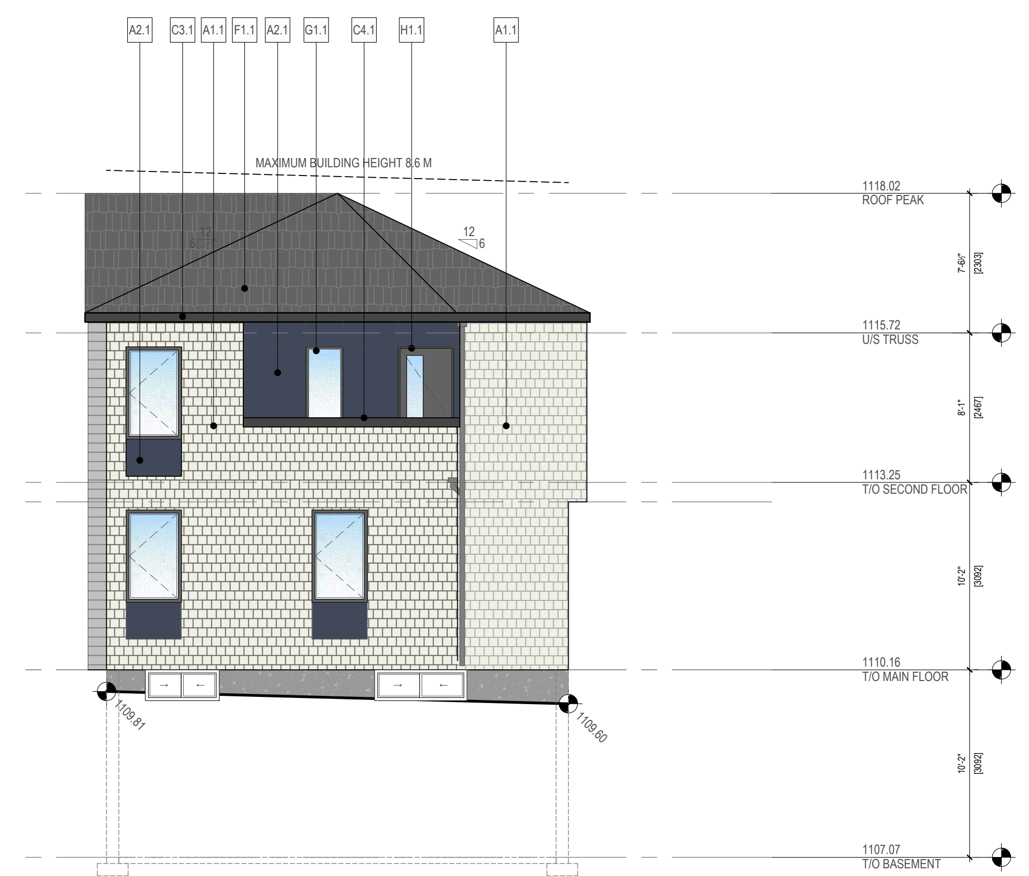
2 BUILDING B - SOUTHWEST ELEVATION DP.402 SCALE: 3/16" = 1'-0"
