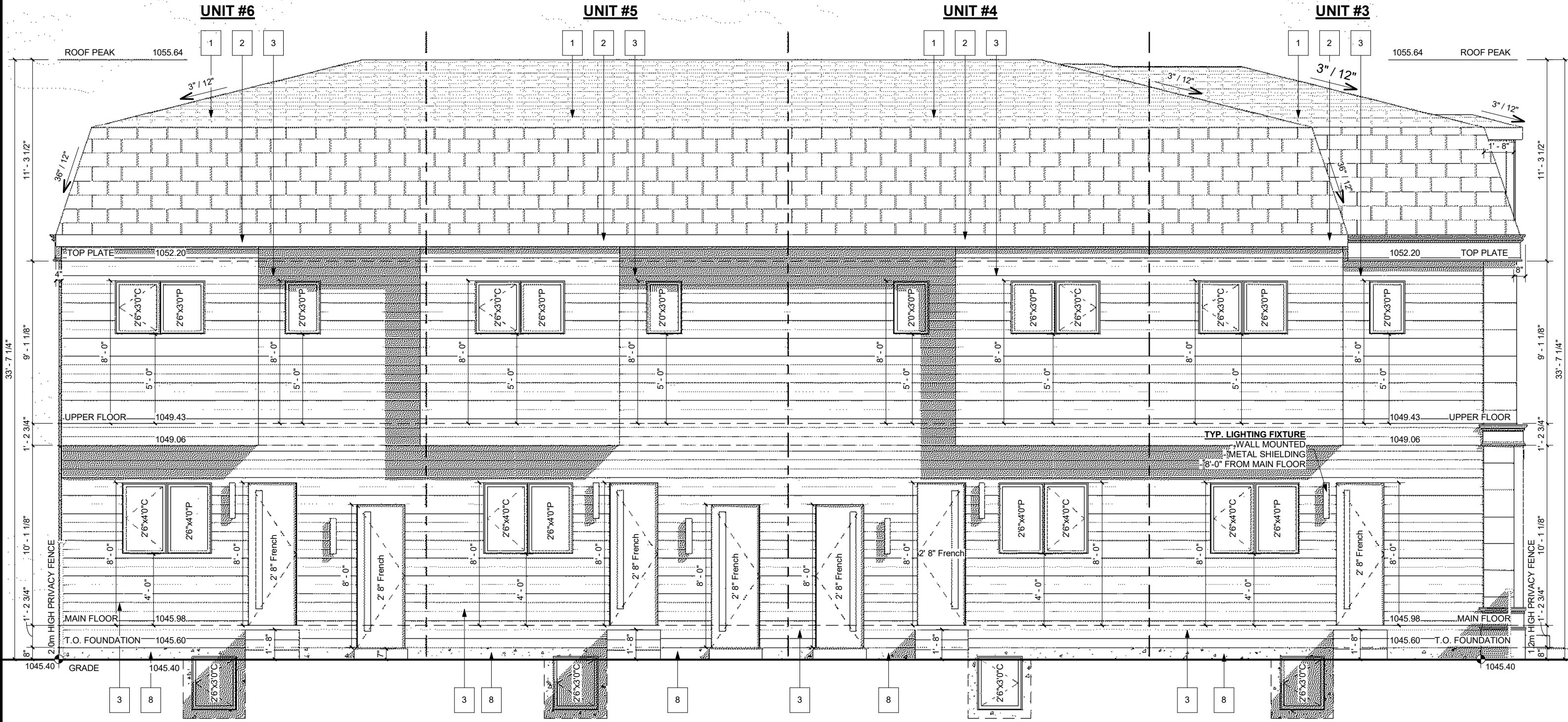
REAR ELEVATION SCALE: 3/16" = 1'-0"
