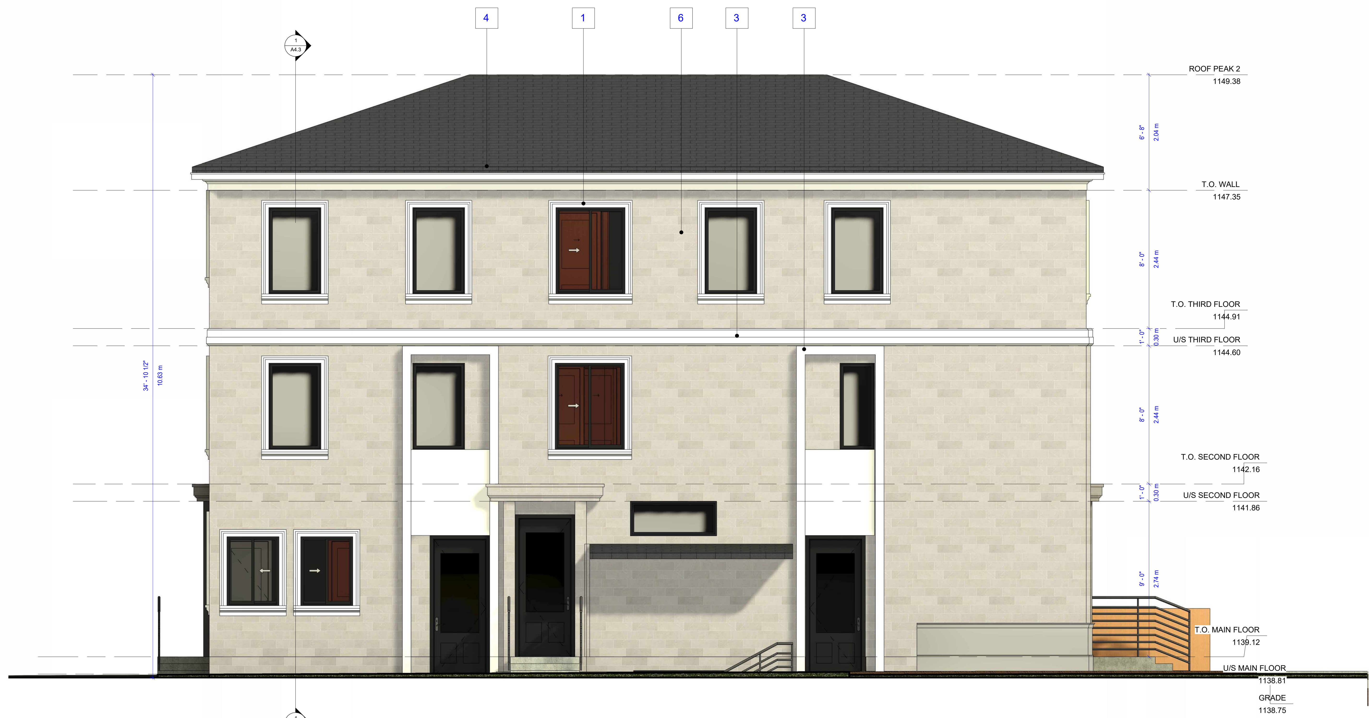
1 BLDG B - NORTH ELEVATION 3/8" = 1'-0"
