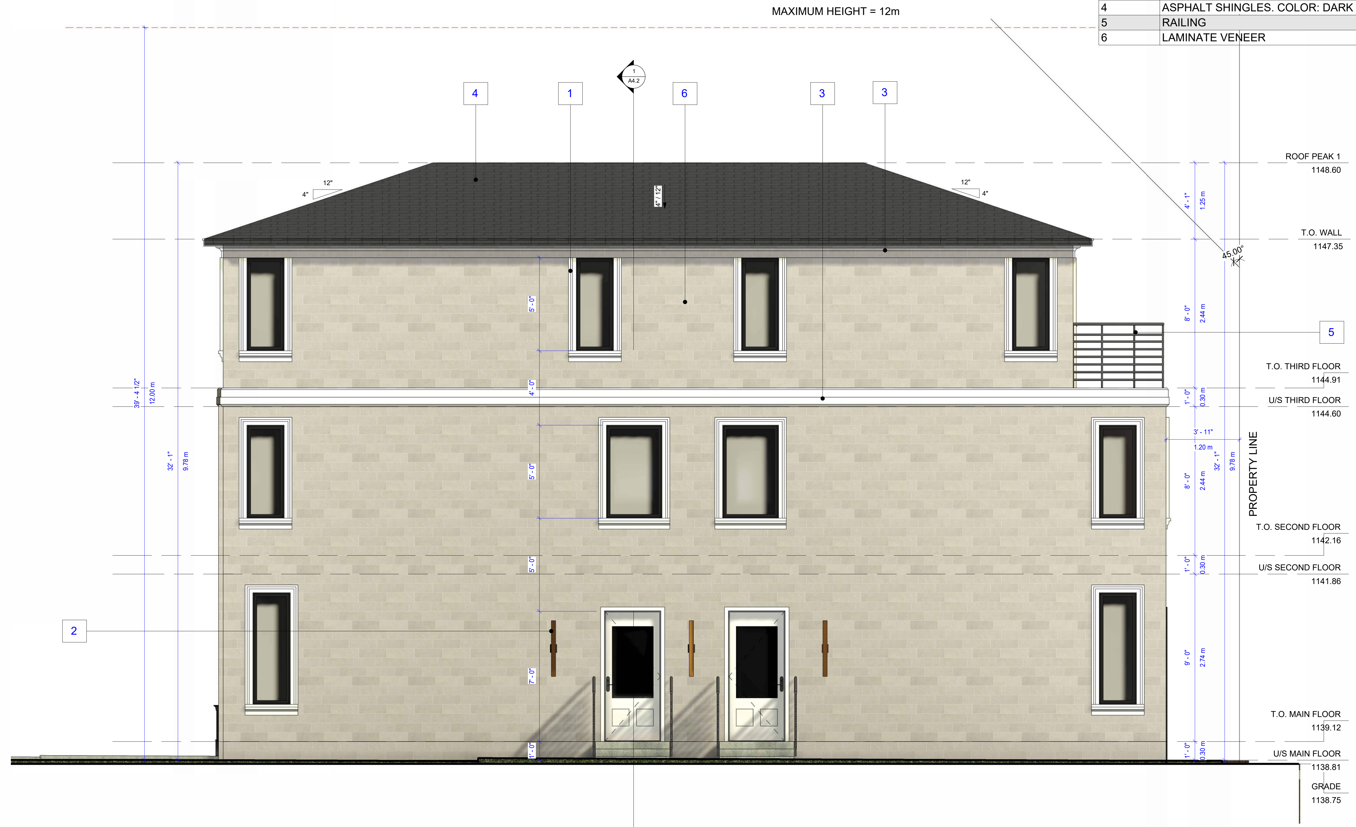
1 BLDG A - SOUTH ELEVATION 3/8" = 1'-0"
