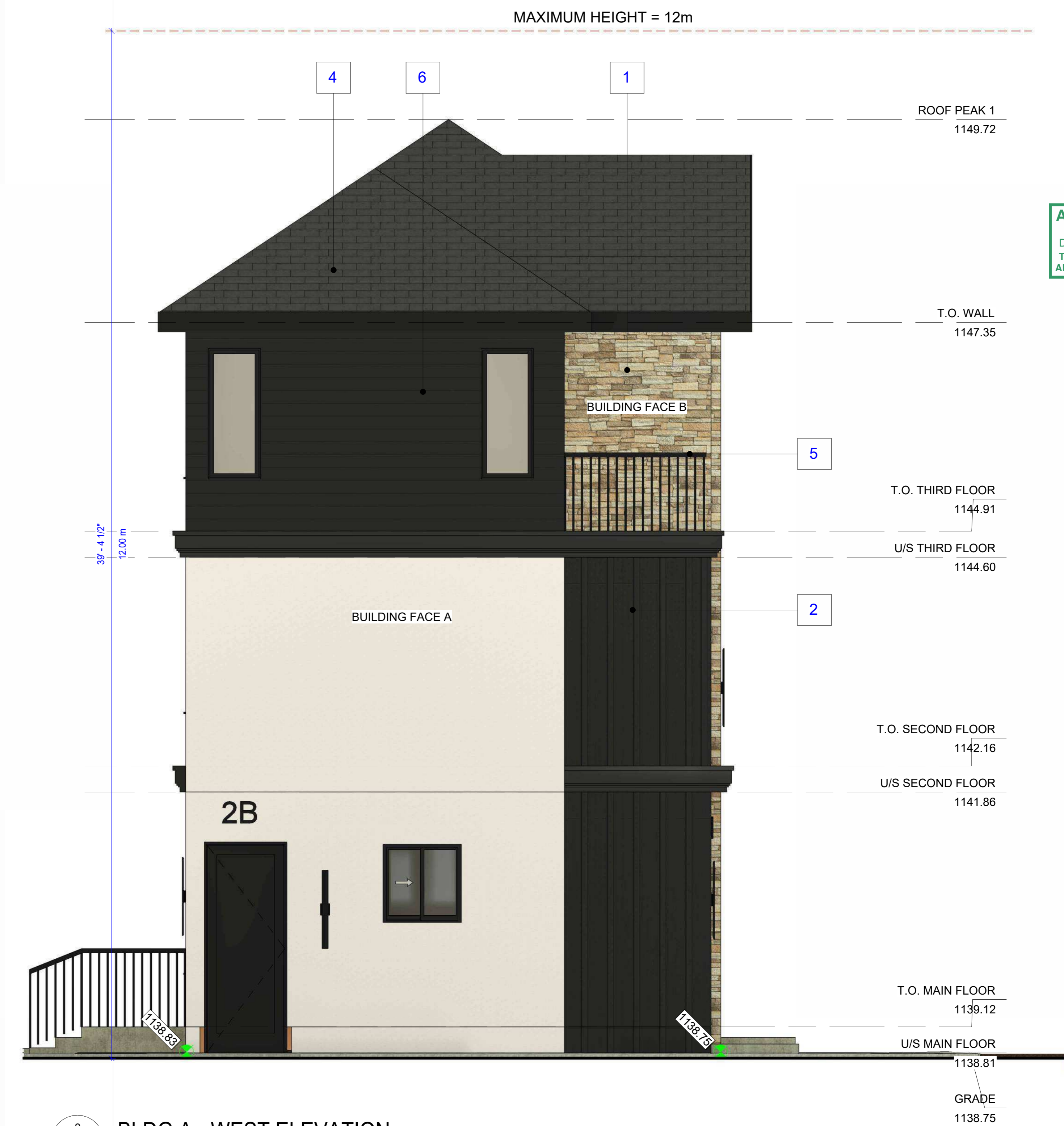
2 BLDG A - WEST ELEVATION 3/8" = 1'-0"
