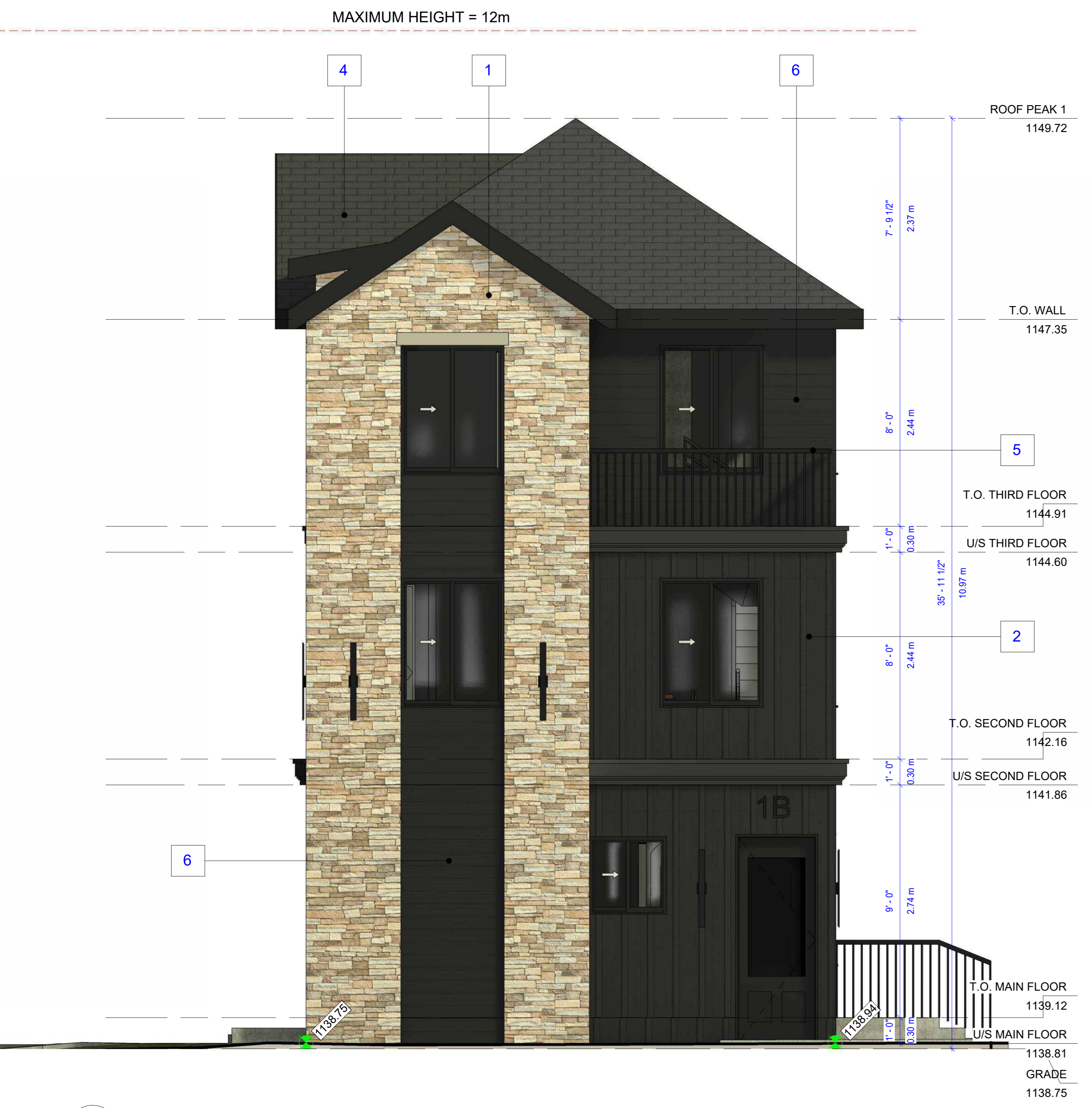
1 BLDG A - EAST ELEVATION 3/8" = 1'-0"
