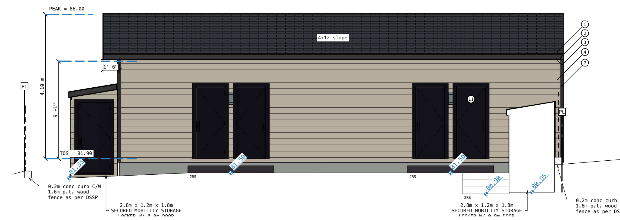
GARAGE ELEVATION (YARD) SCALE: 3/16"=1'-0"
