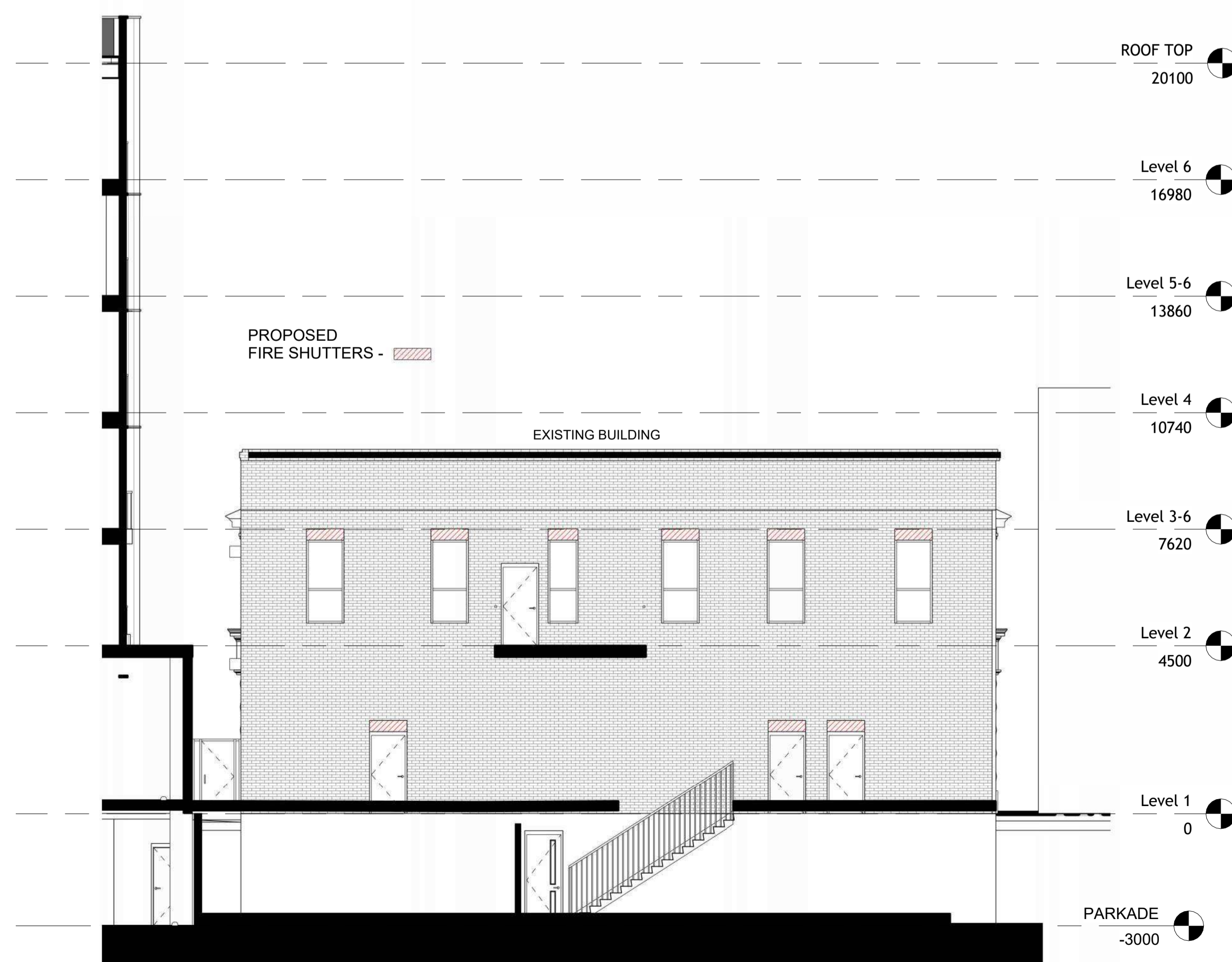
4 CARSON BLOCK - NORTH ELEVATION DPO.02 1:100
