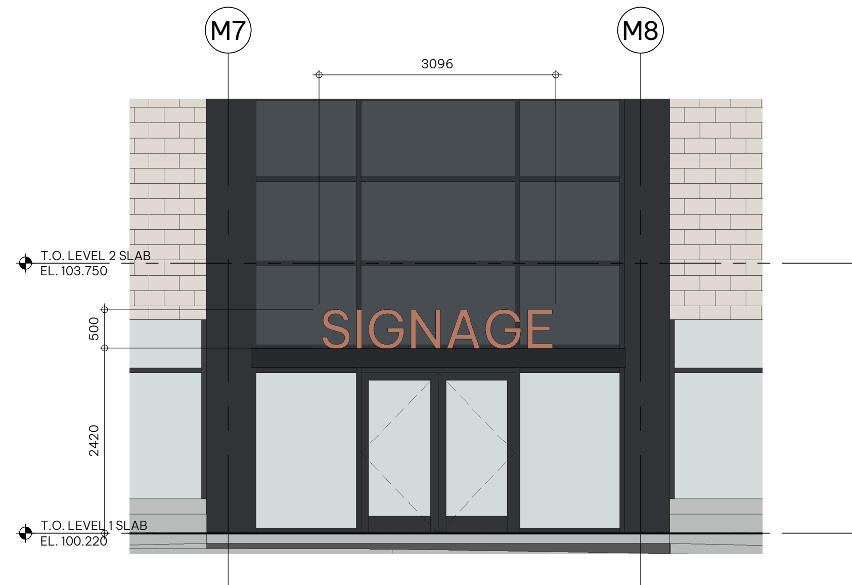
1 Front Entry Signage DP4.00 | DP1.05 SCALE: 1:50
