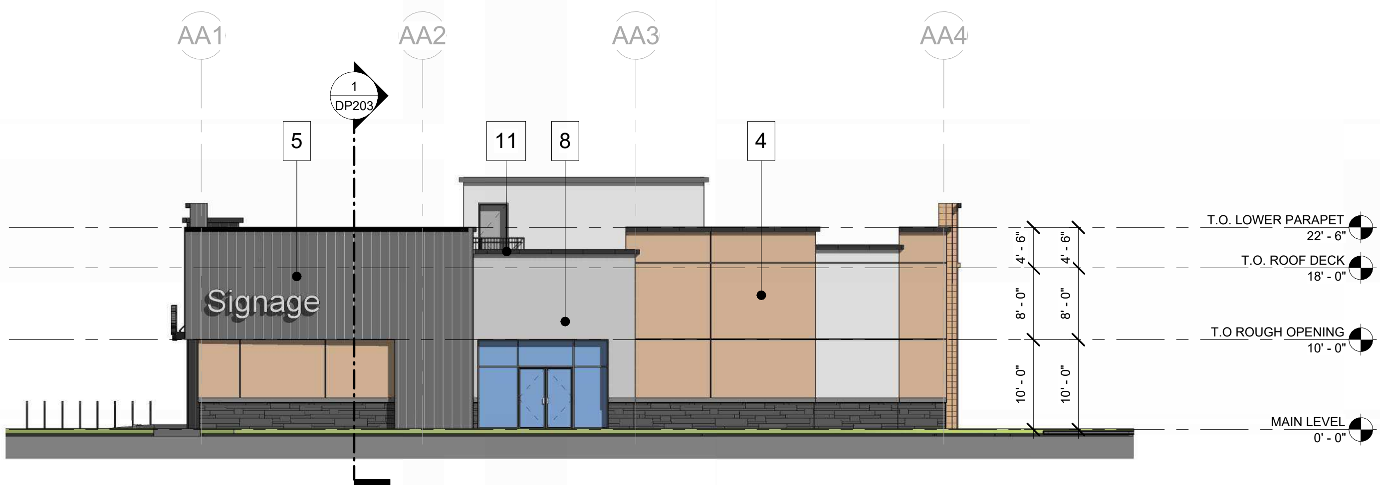
3 BUILDING A - SIDE ELEVATION (EAST) DP202 3/32" = 1'-0"
