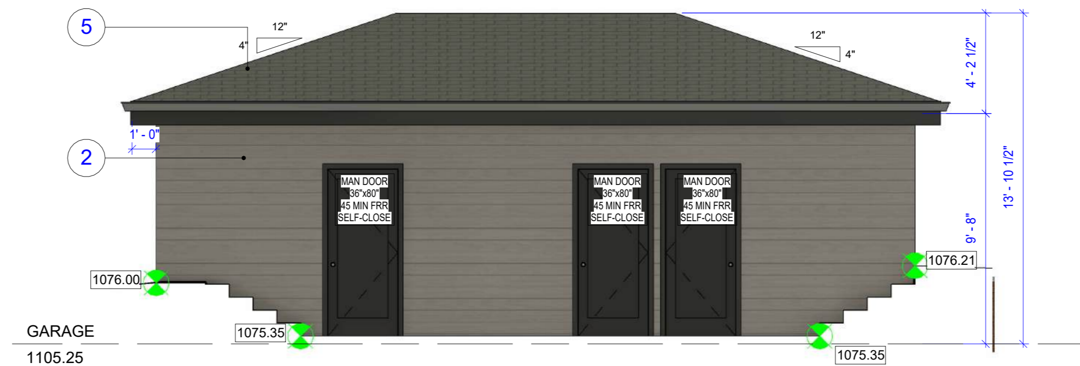
3 GARAGE REAR ELEVATION A3.5 1/4" = 1'-0"
