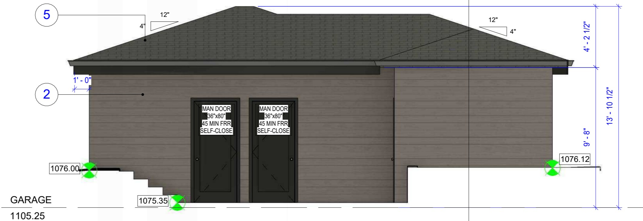
3 GARAGE REAR ELEVATION A3.5 1/4" = 1'-0"
