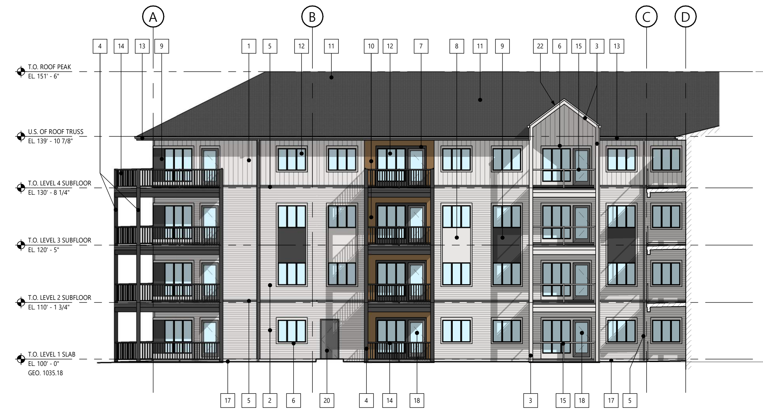
3 | SOUTH COURTYARD ELEVATION DPA.01 | SCALE: 3/32" = 1'-0"
