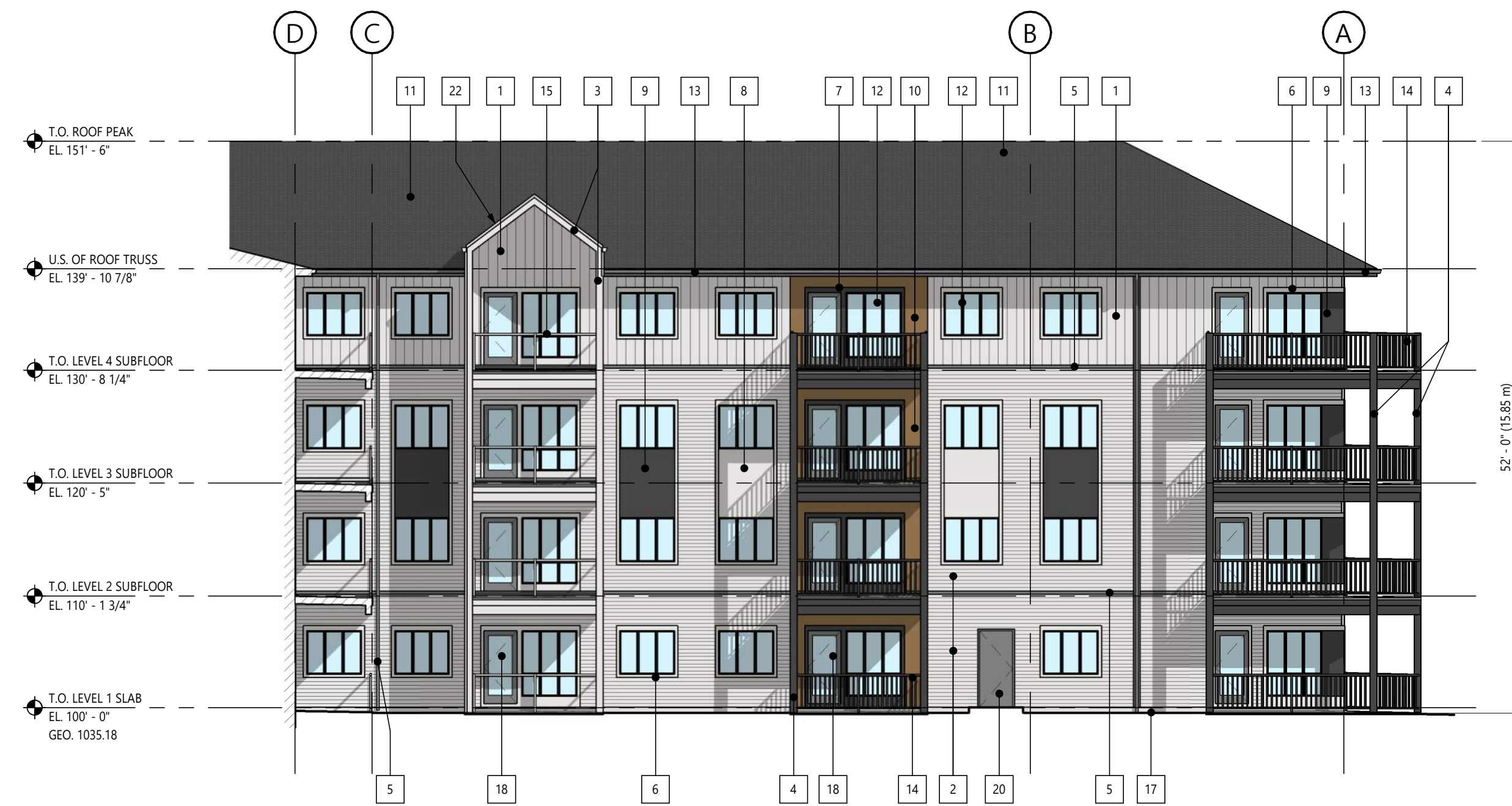
2 | NORTH COURTYARD ELEVATION DPA.01 | SCALE: 3/32" = 1'-0"
