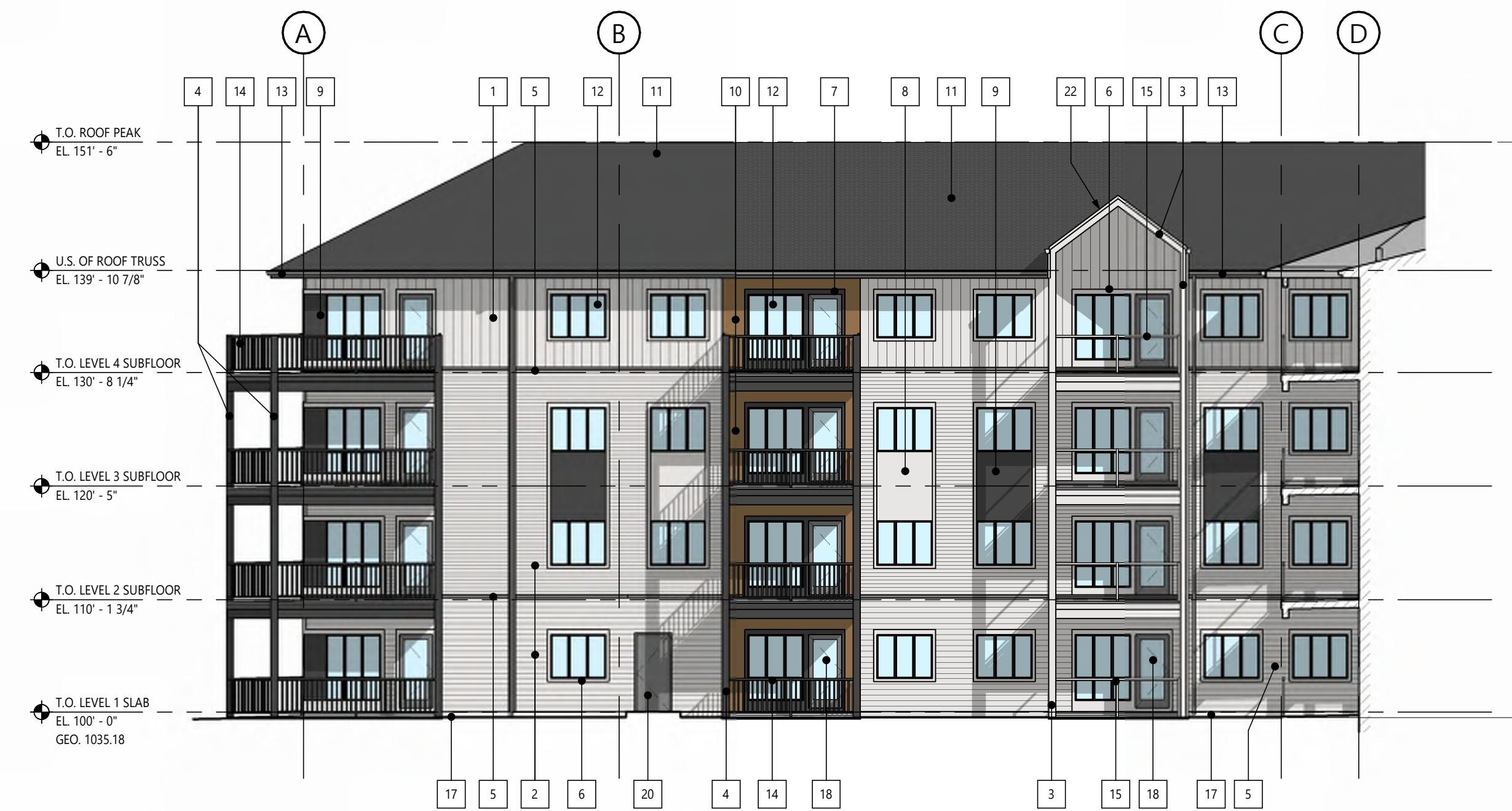
3 | SOUTH COURTYARD ELEVATION DP4.01 | SCALE: 3/32" = 1'-0"
