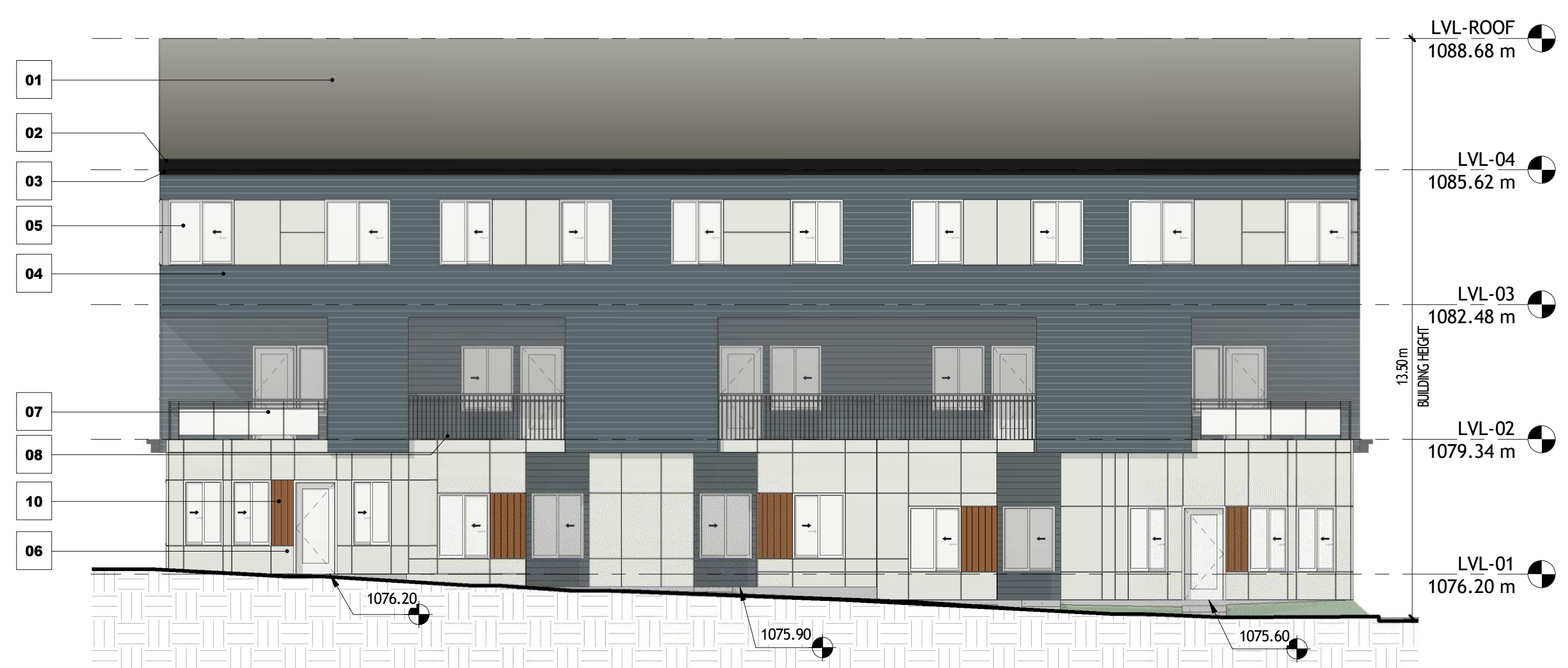
5 BUILDING 06 - EAST ELEVATION 1 : 100
