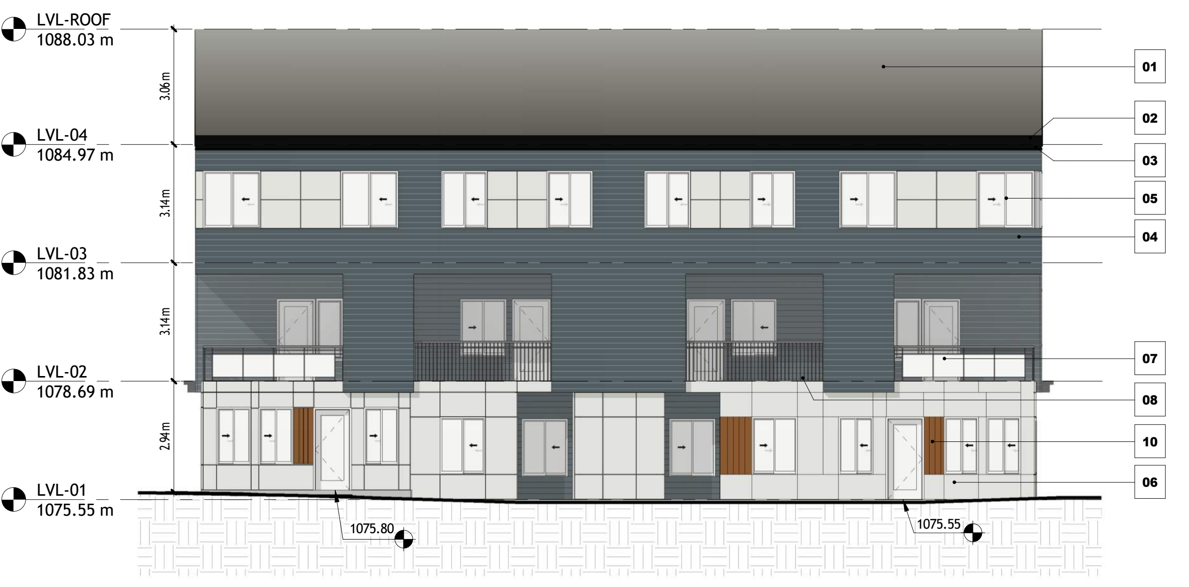
5 BUILDING 02 - EAST ELEVATION 1 : 100
