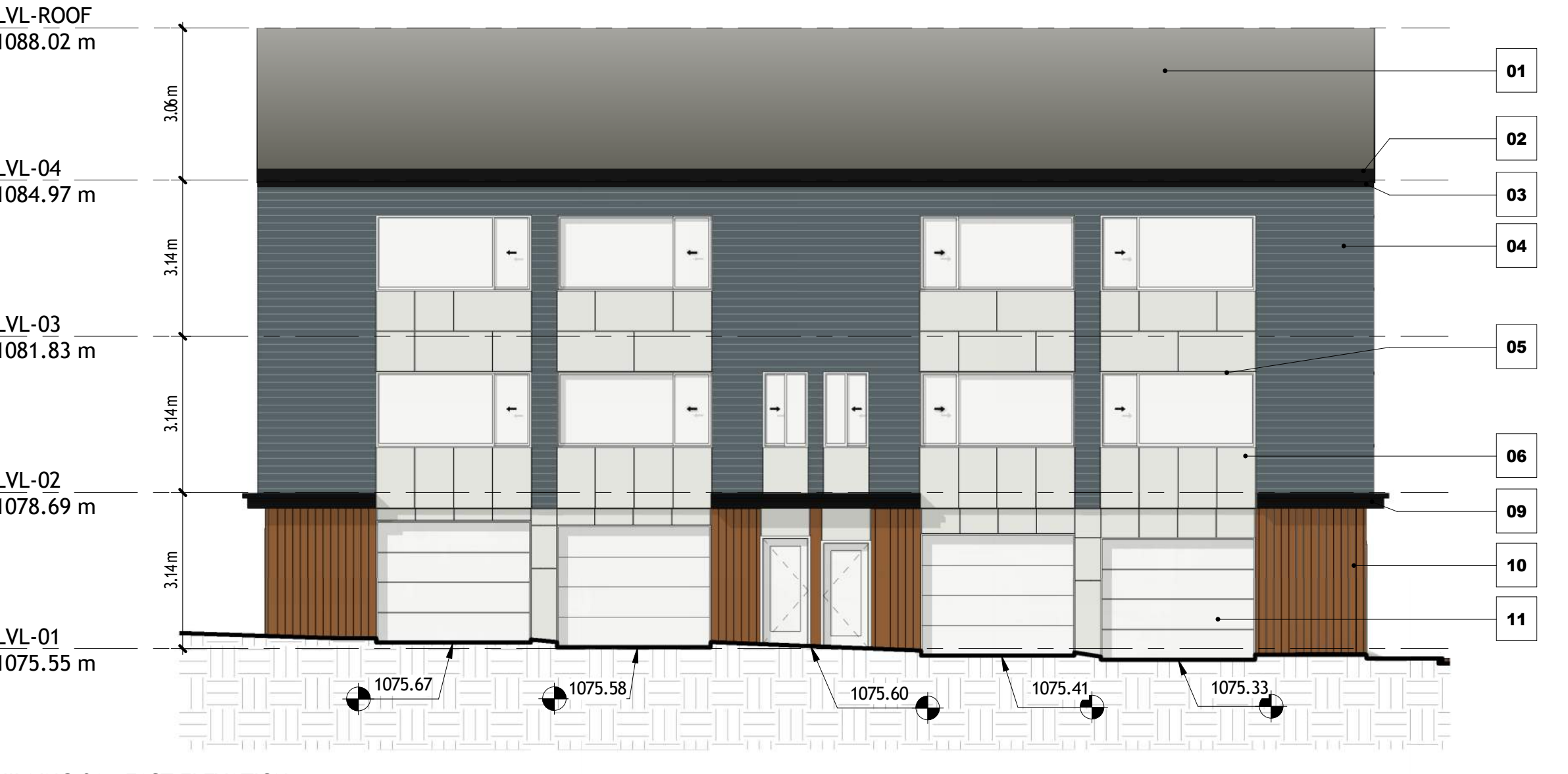
1 BUILDING 01 - EAST ELEVATION 1 : 100
