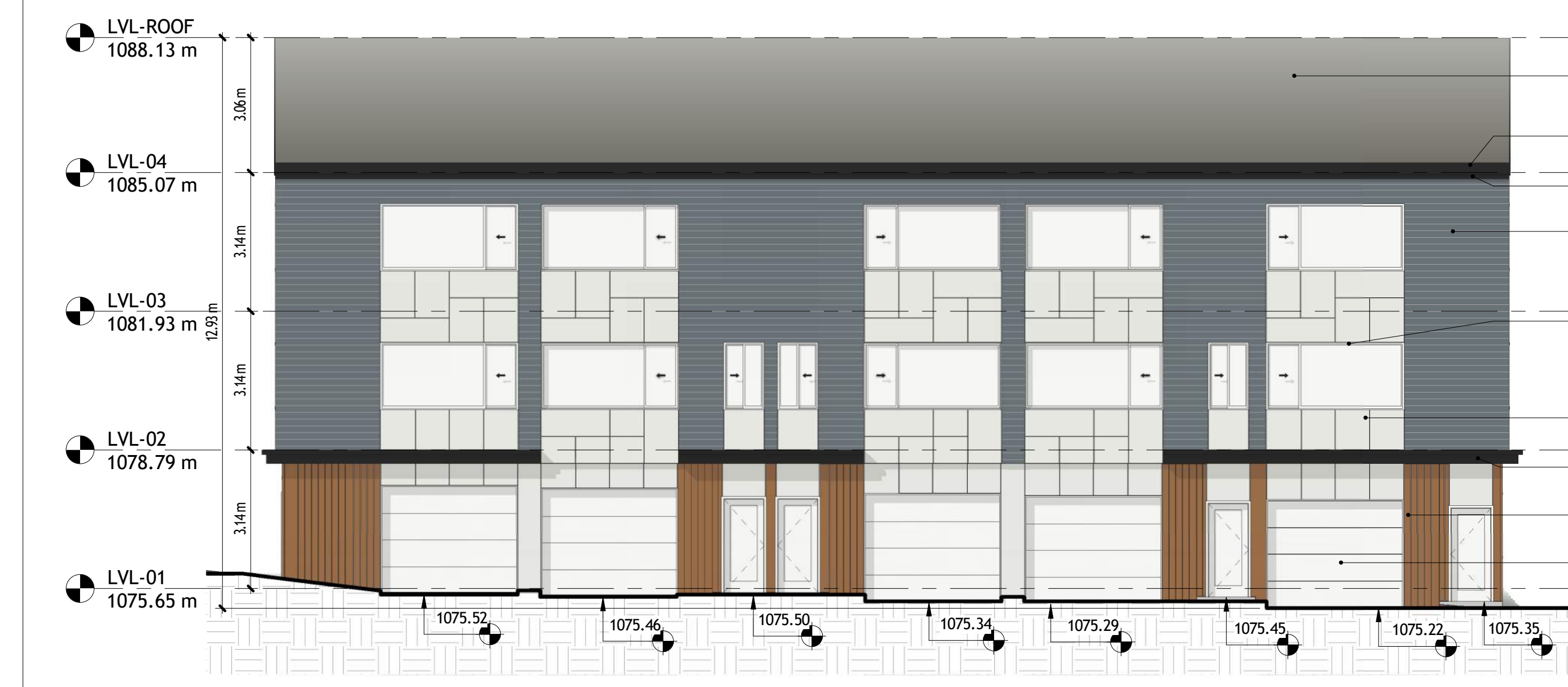
1 BUILDING 05 - EAST ELEVATION 1 : 100
