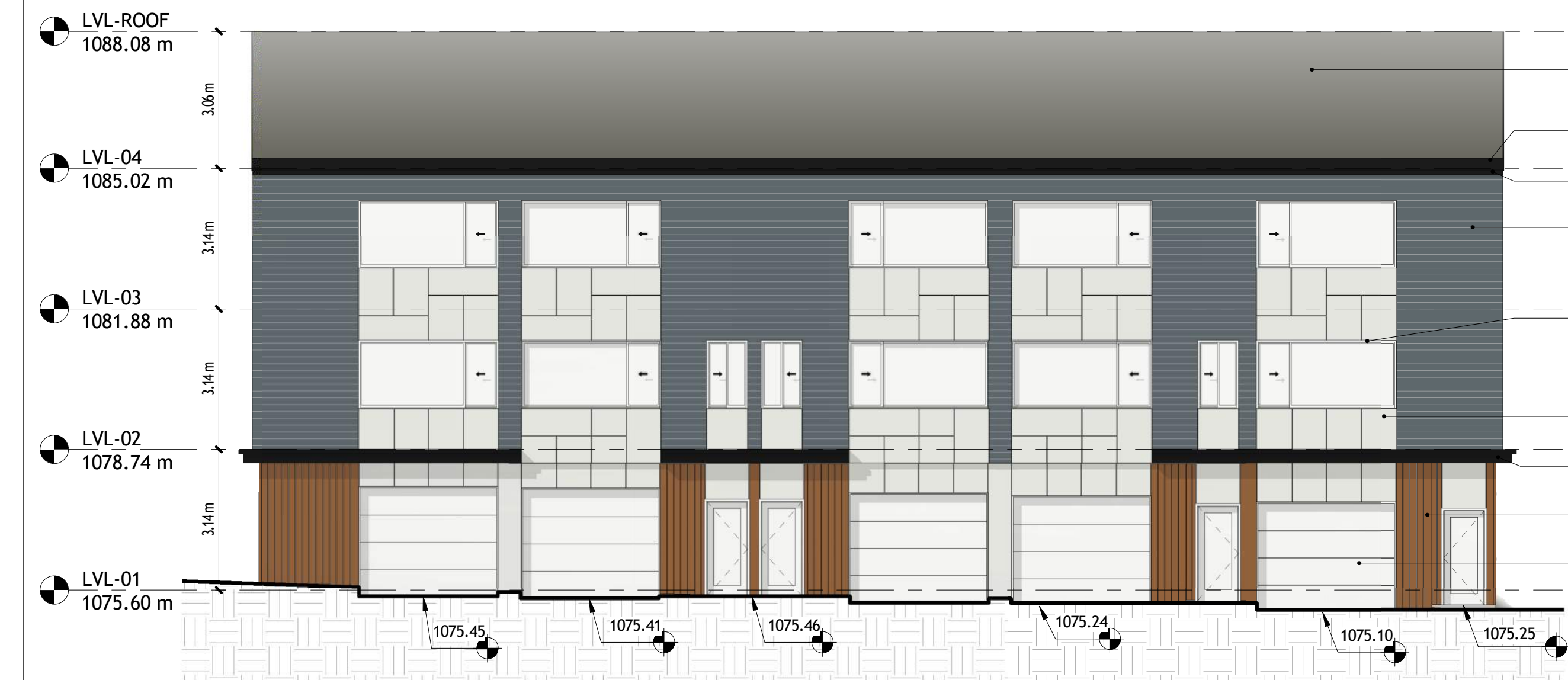
1 BUILDING 03 - EAST ELEVATION 1 : 100
