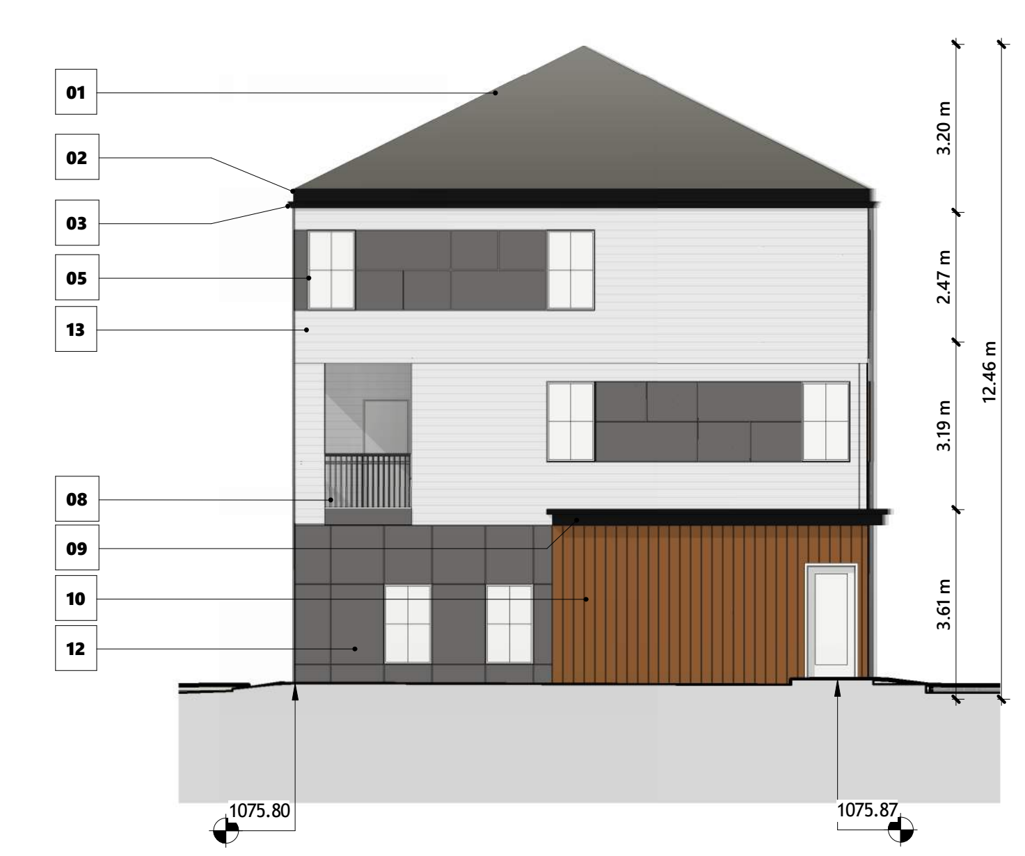
3 BUILDING 01 - SOUTH ELEVATION 1 : 100
