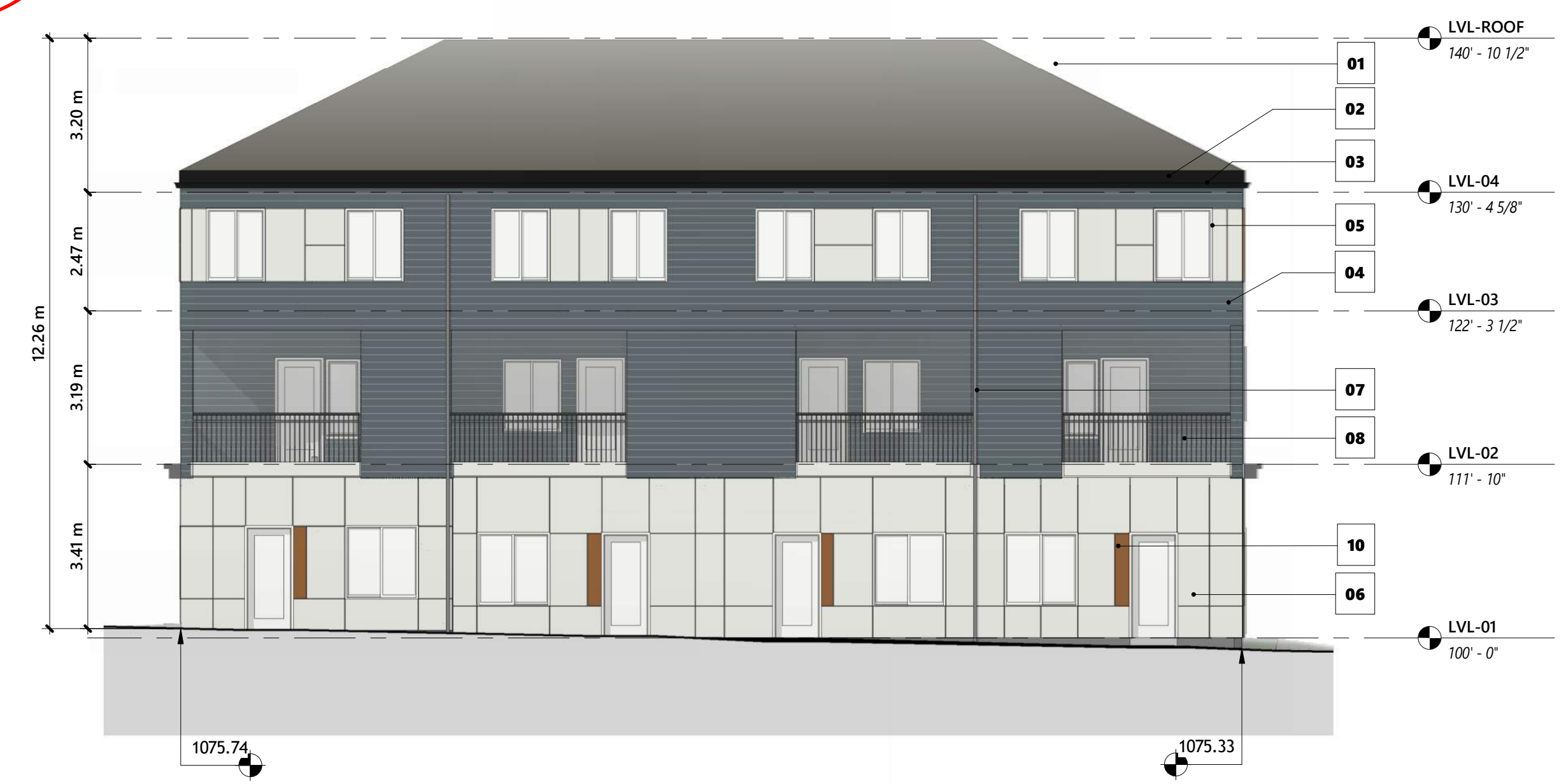
5 BUILDING 02 - EAST ELEVATION 1 : 100
