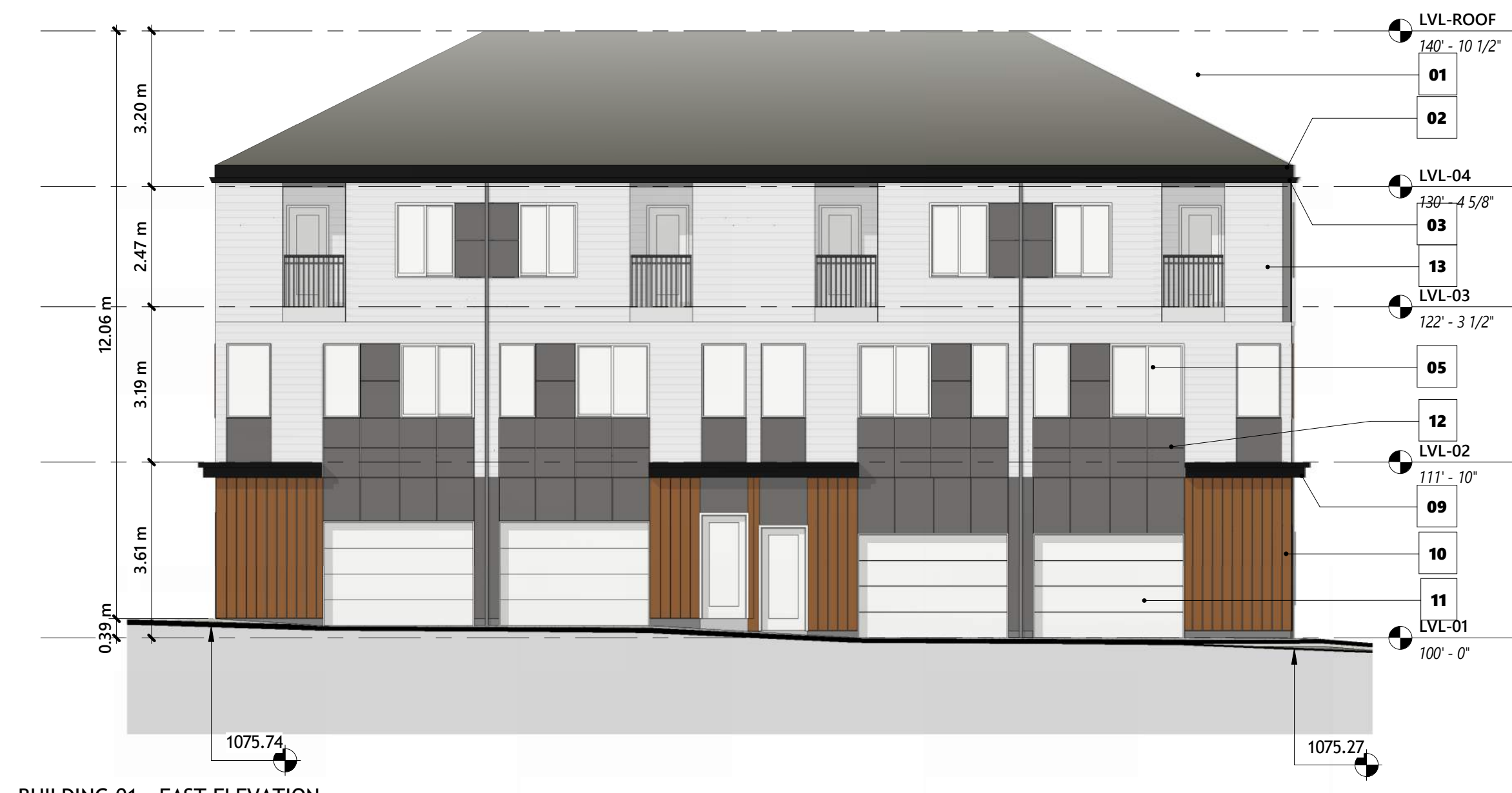
1 BUILDING 01 - EAST ELEVATION 1 : 100
