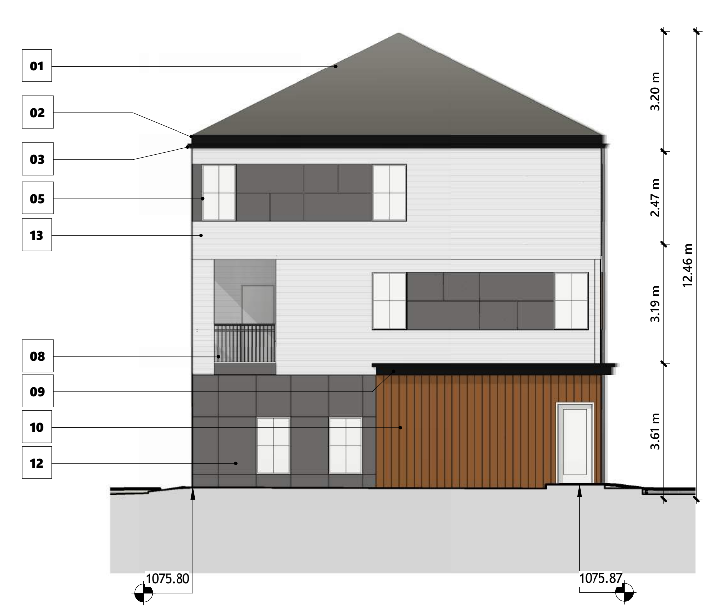
3 BUILDING 01 - SOUTH ELEVATION 1 : 100
