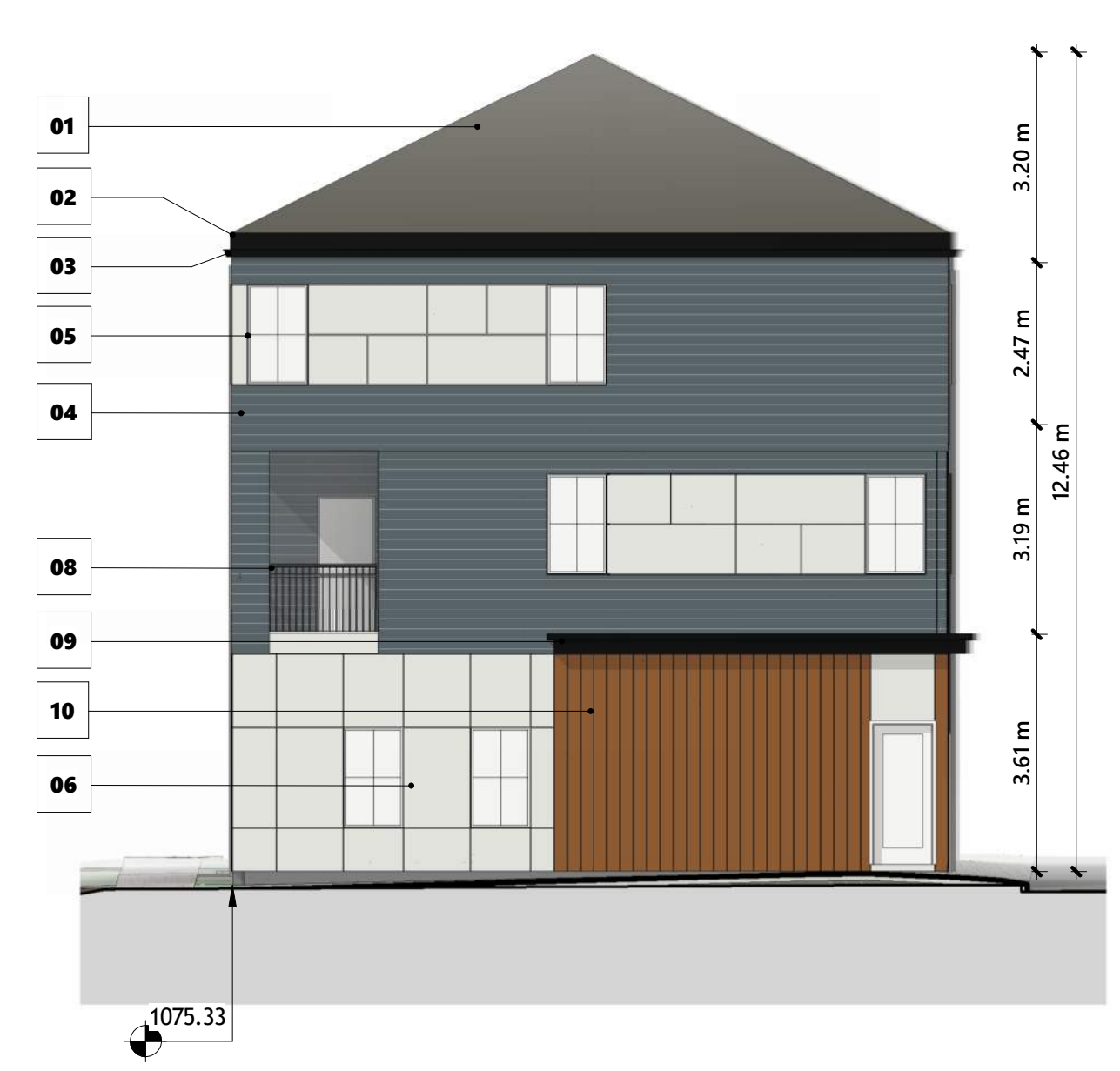
7 BUILDING 02 - NORTH ELEVATION 1 : 100
