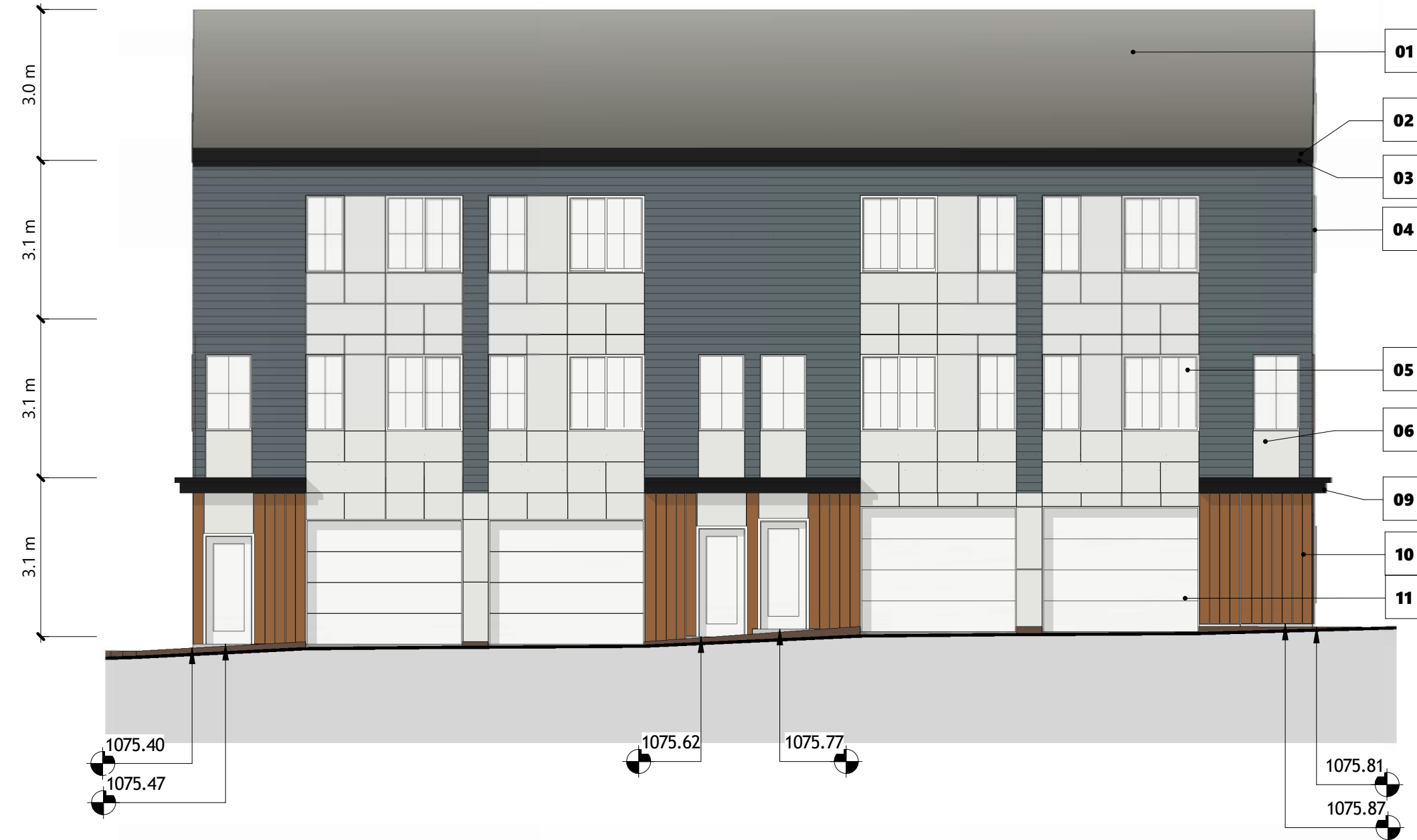
6 BUILDING 02 - WEST ELEVATION 1 : 100
