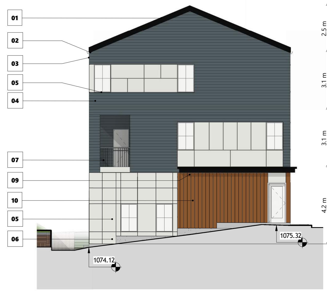
4 BUILDING 08 0 WEST ELEVATION 1 : 100
