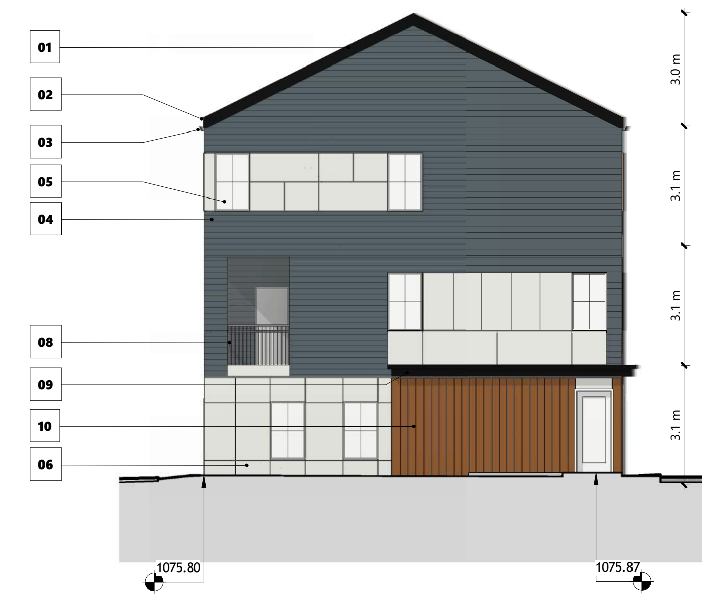
3 BUILDING 01 - SOUTH ELEVATION 1 : 100
