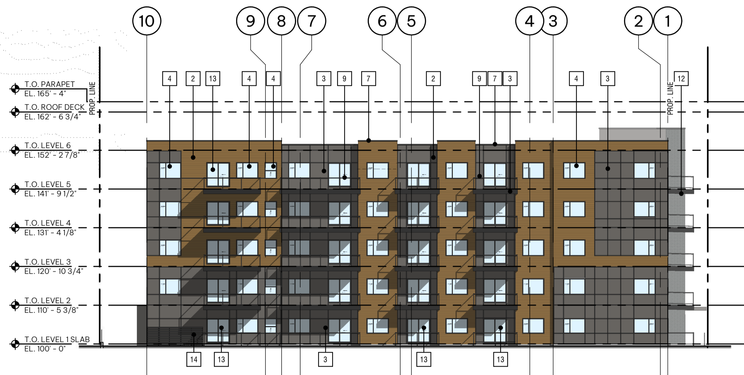
4 Building B East Elevation
