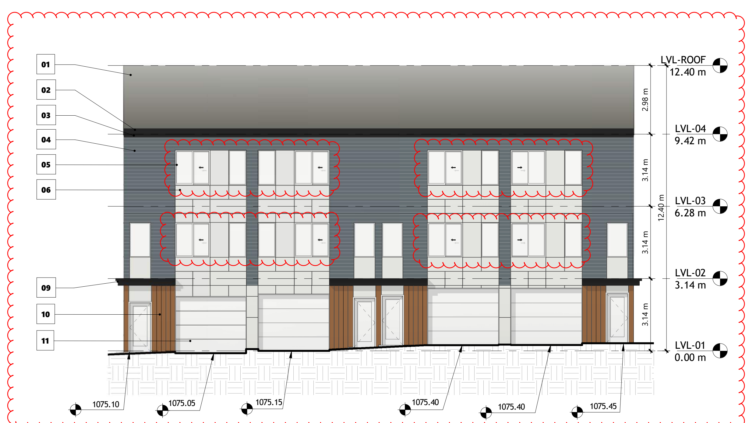
8 BUILDING 02 - WEST ELEVATION 1 : 100
