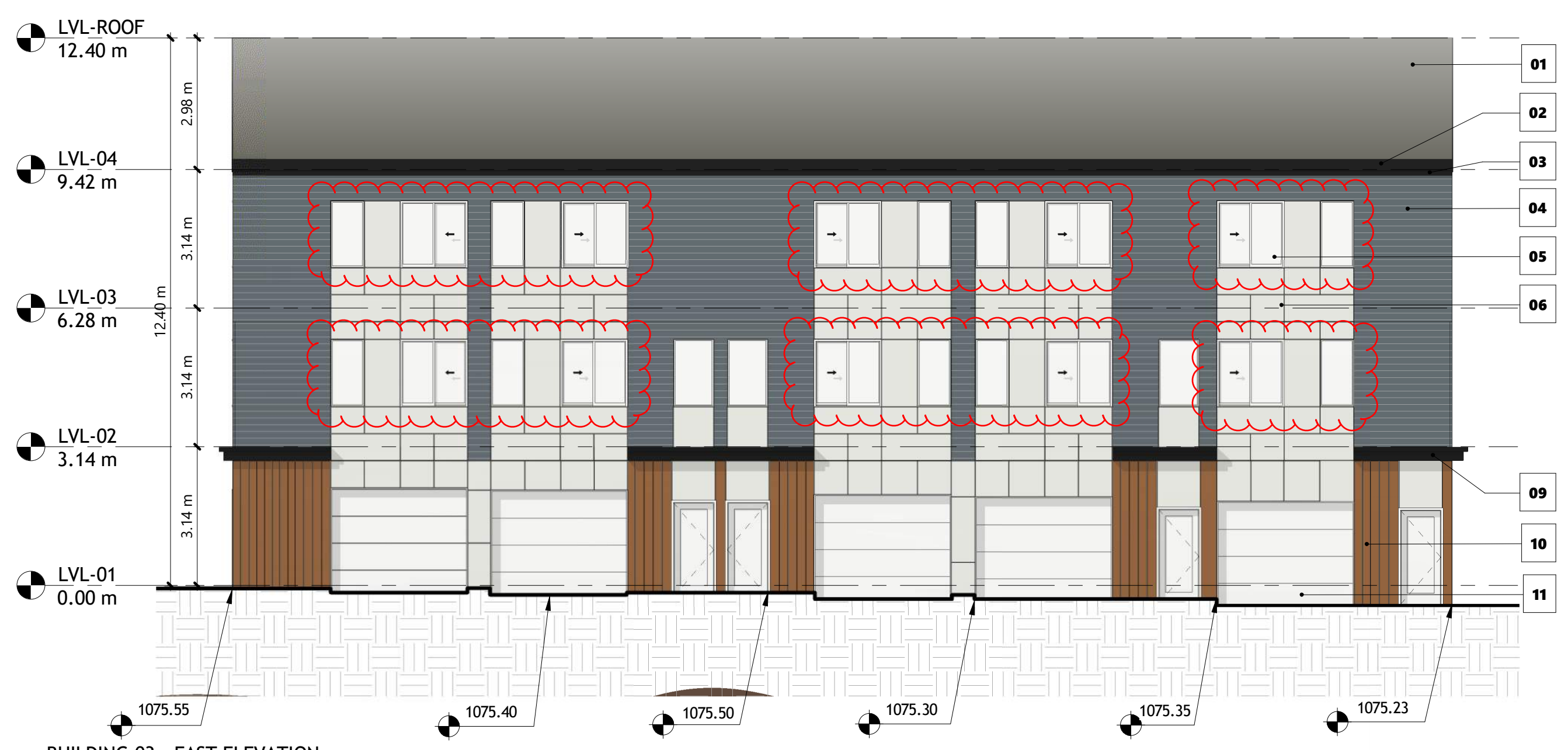
1 BUILDING 03 - EAST ELEVATION 1 : 100
