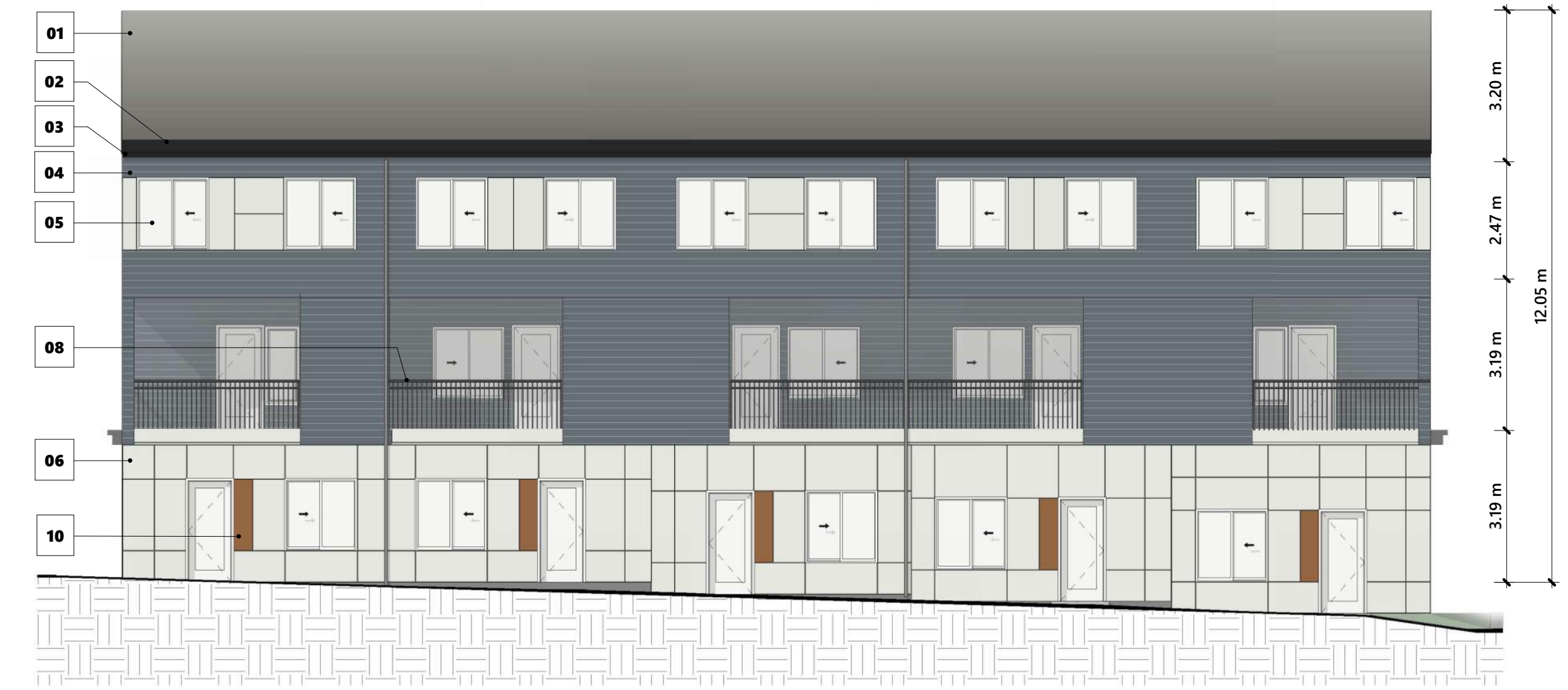
7 BUILDING 08 - EAST ELEVATION 1 : 100
