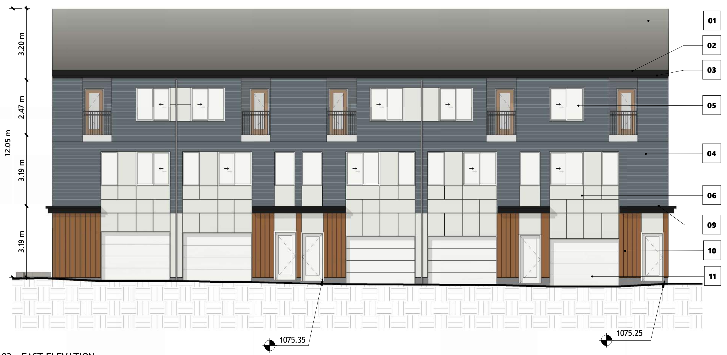
1 BUILDING 03 - EAST ELEVATION 1 : 100
