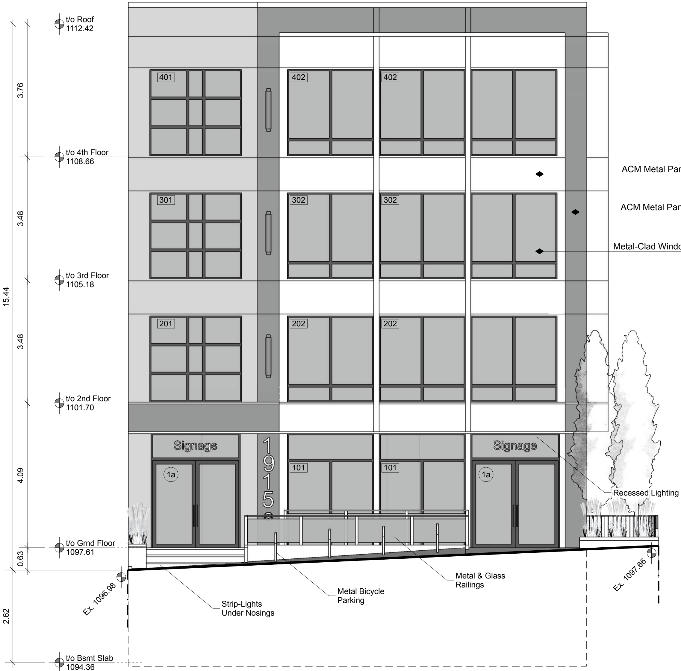
1 North Elevation A3.1 3/16" = 1'0
