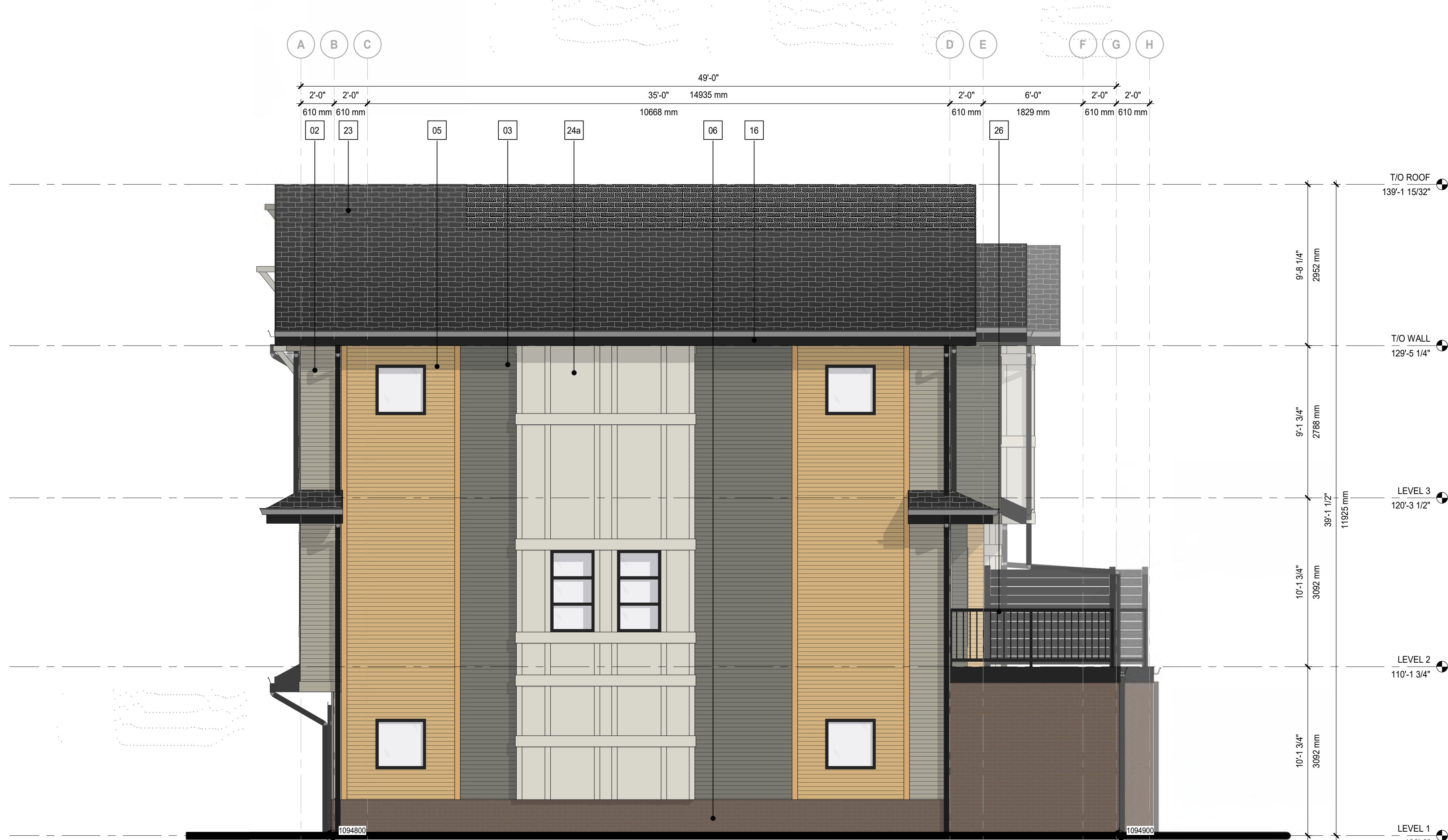
1 Left Elevation TH D DR40-D-03 SCALE: 1:50
