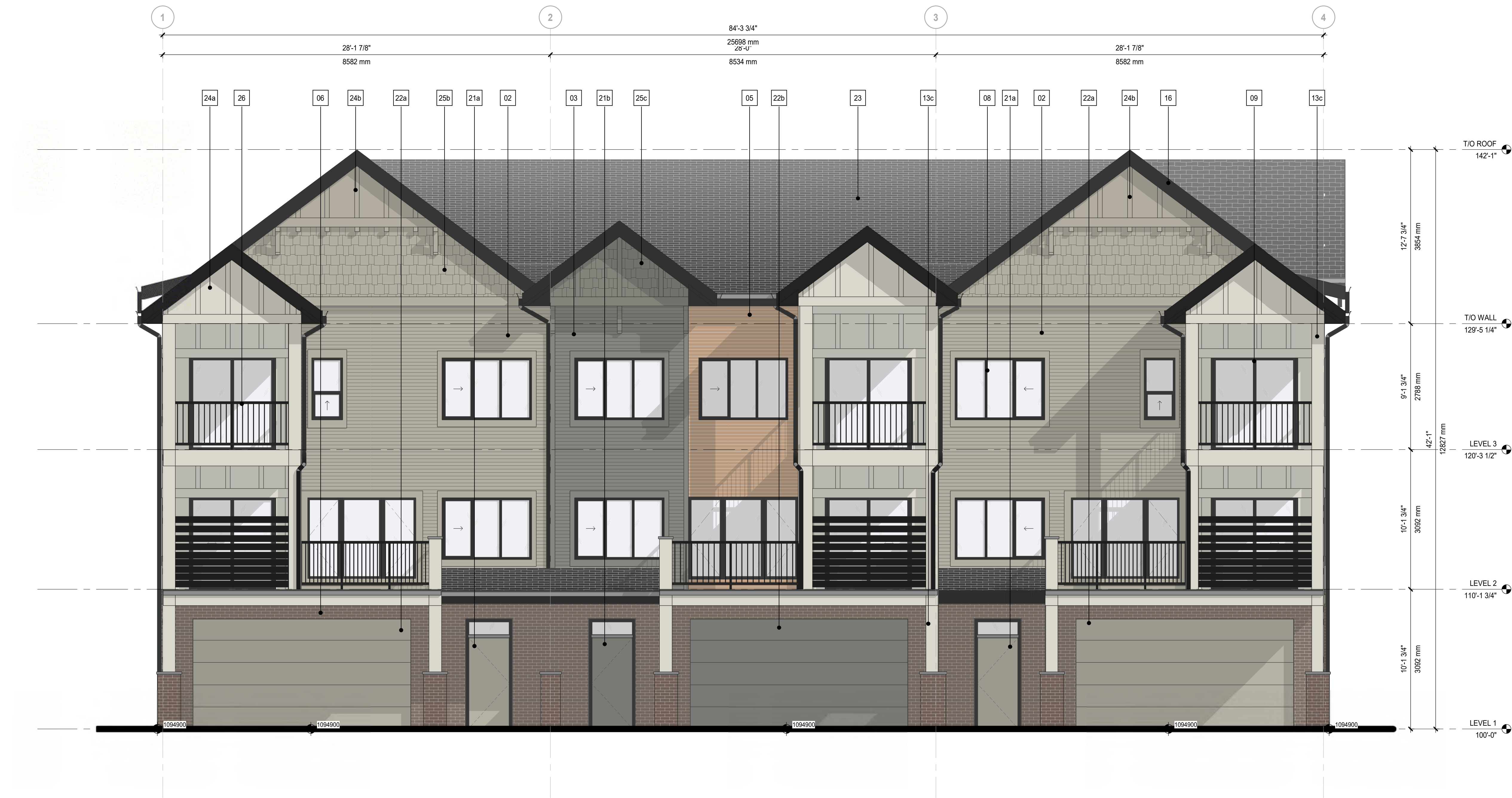
1 Front Elevation A - TH P DP40-P-01 SCALE: 1:50
