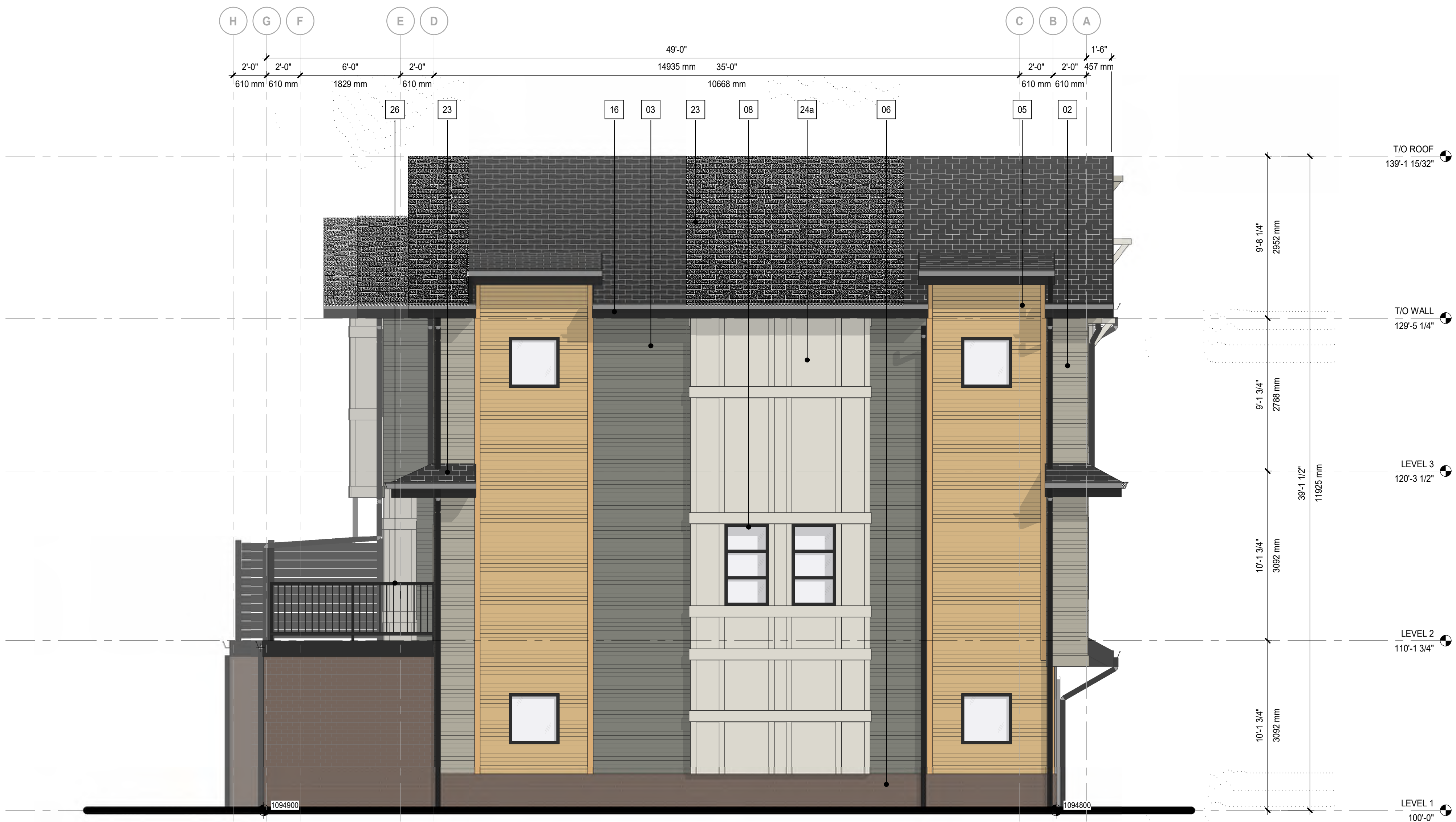
1 Left Elevation TH D DR40-D-03 SCALE: 1:50
