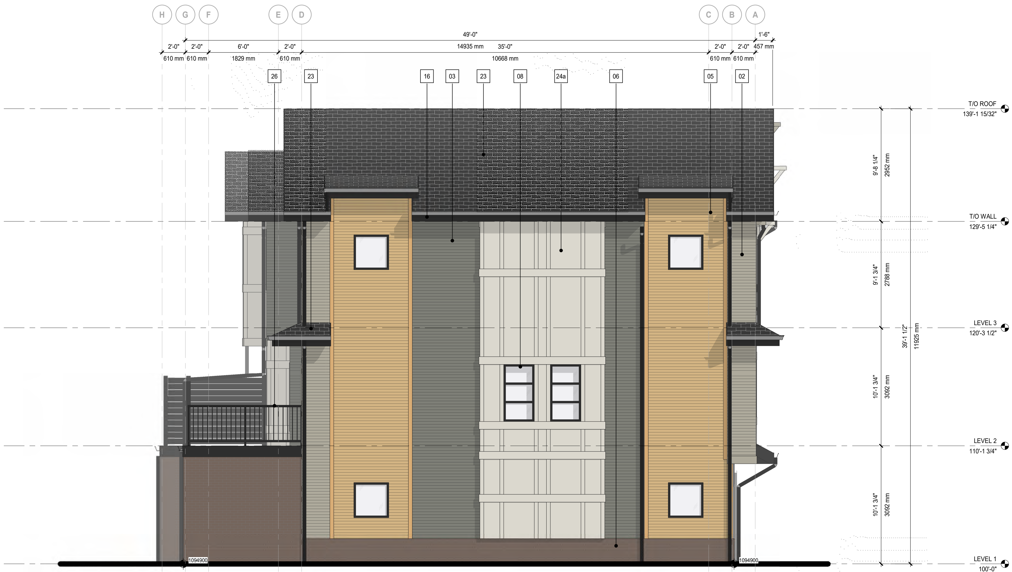
1 Left Elevation TH G DWG-G-03 SCALE: 1:50
