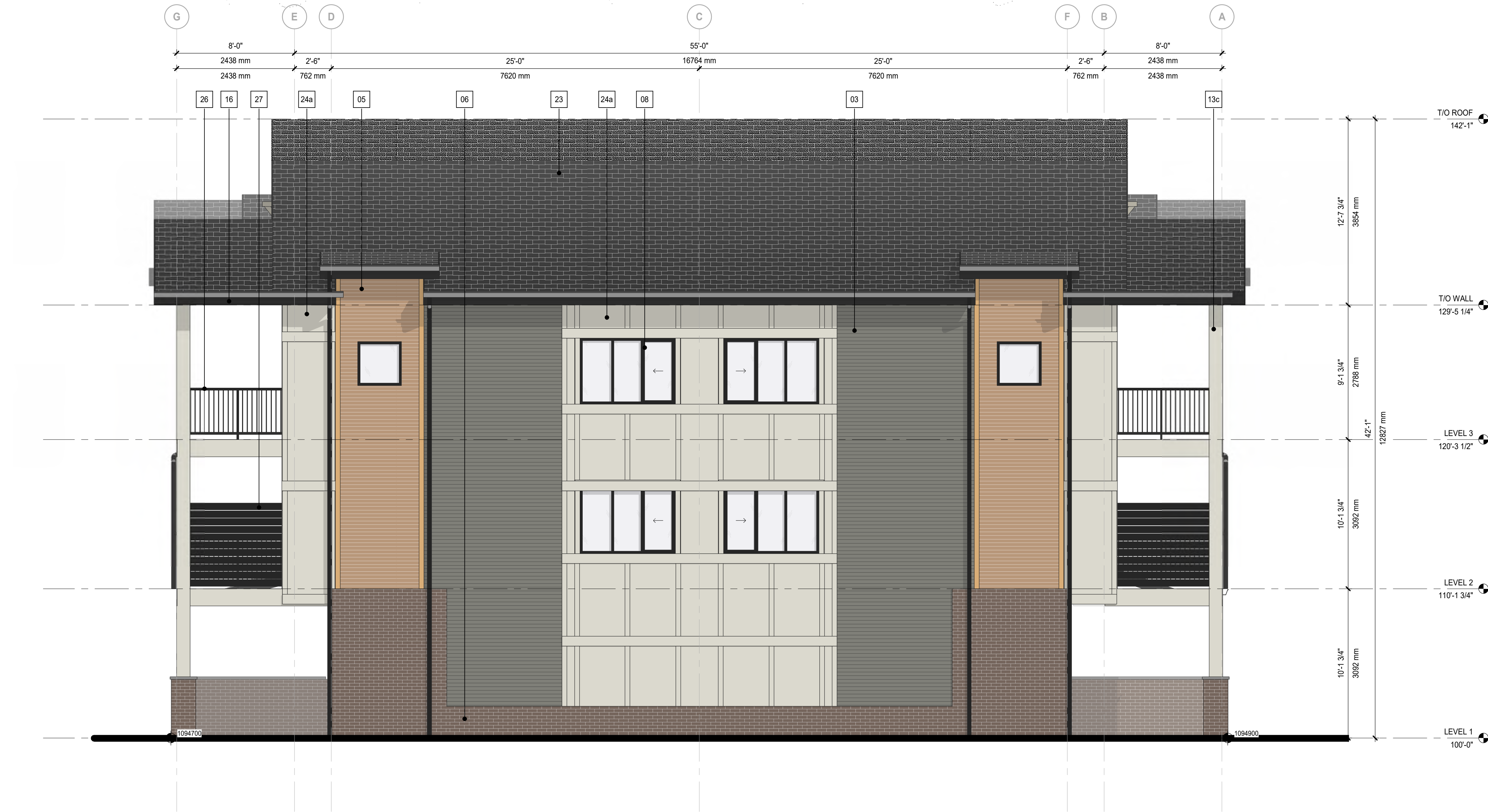
2 Side Elevation Blind - TH P DP40-P-02 SCALE: 1:50
