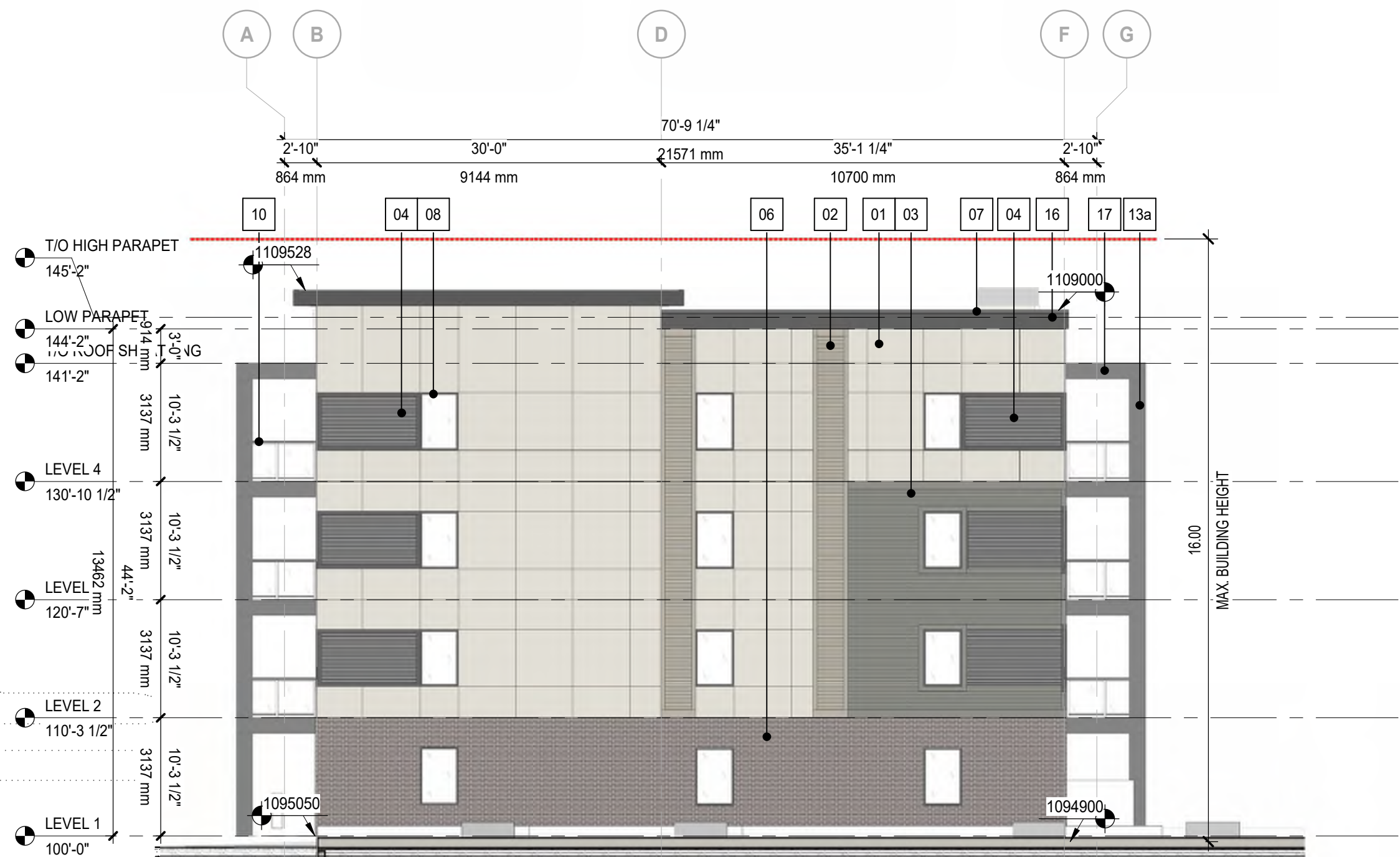
2 BLDG 6000 - SOUTH ELEVATION DP40-02-08 SCALE: 1:125
