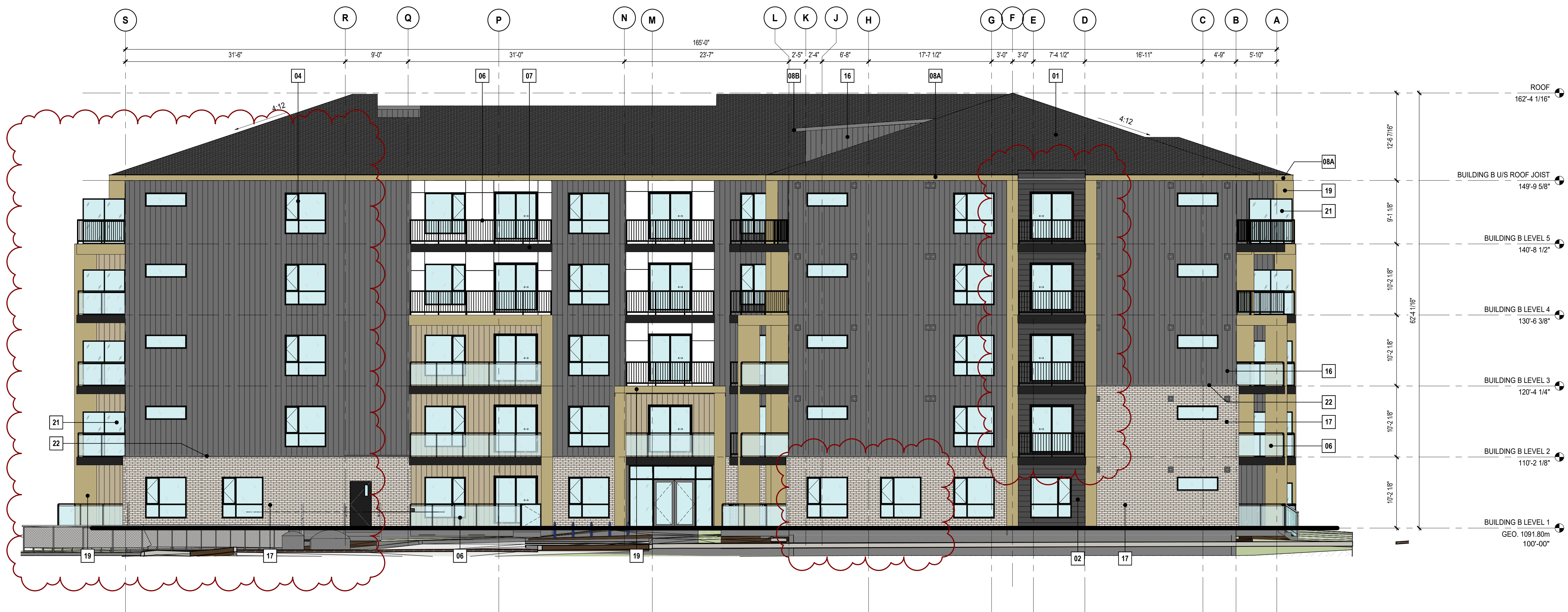
1 DP_A40 OVERALL BUILDING A ELEVATION - WEST SCALE: 1/8" = 1'-0"
