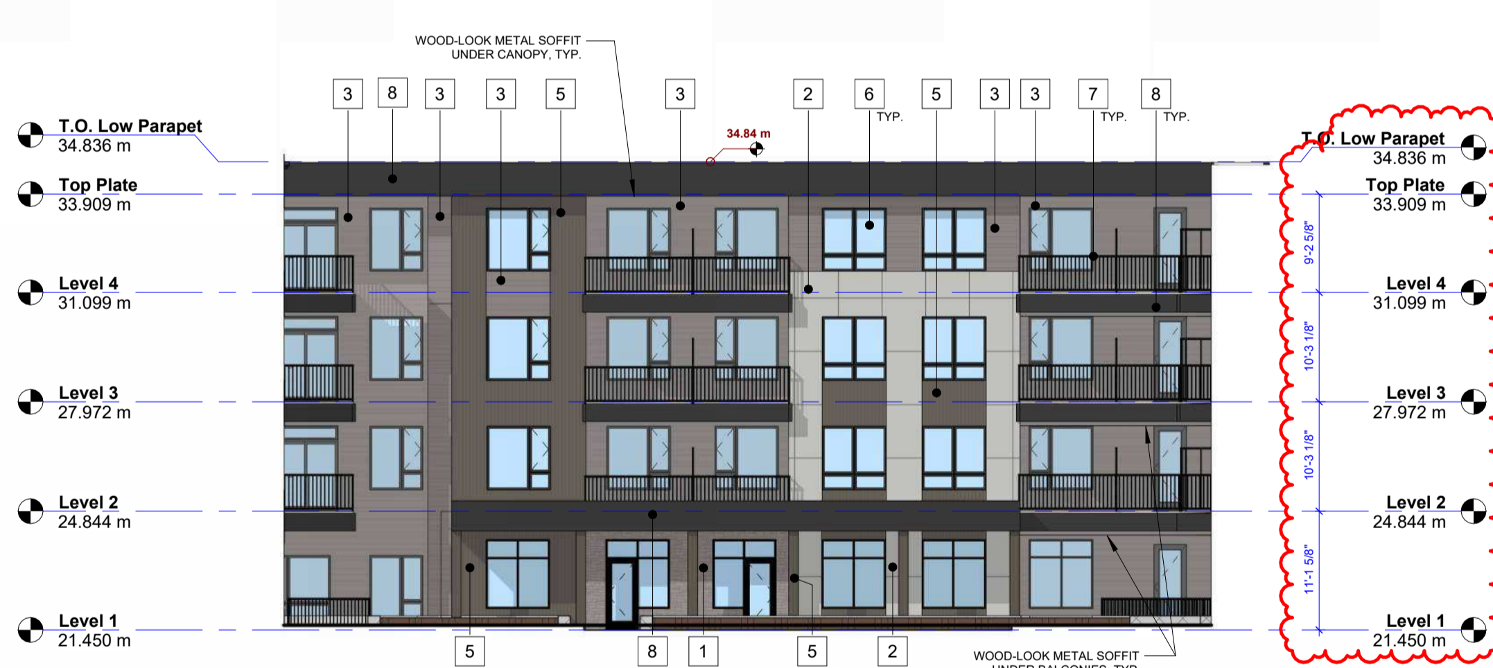
3 South Elevation - Courtyard 2/25" = 1'-0"
