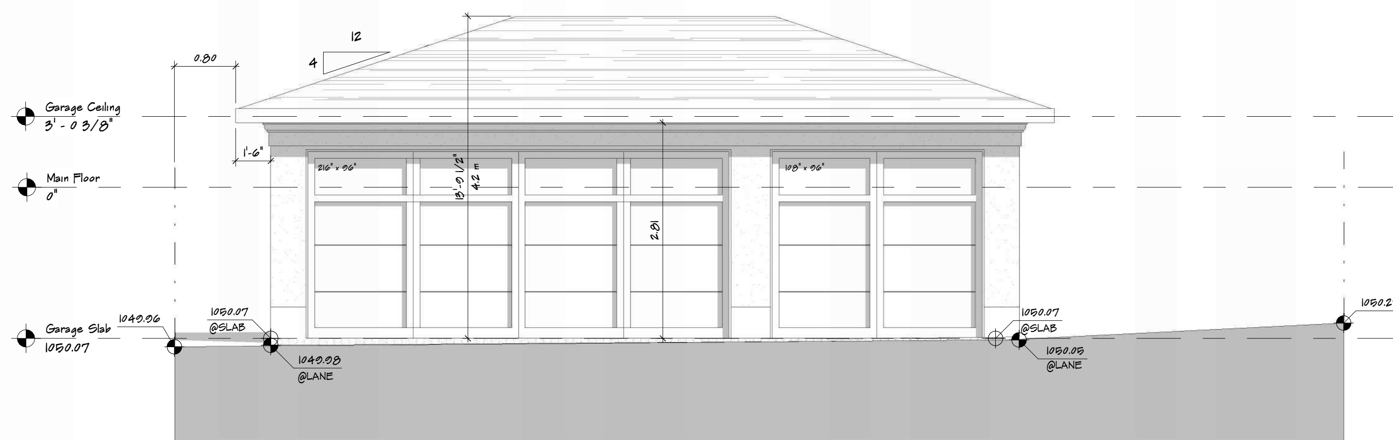
3 Garage Rear Elevation A5 1/4" = 1'-0"
