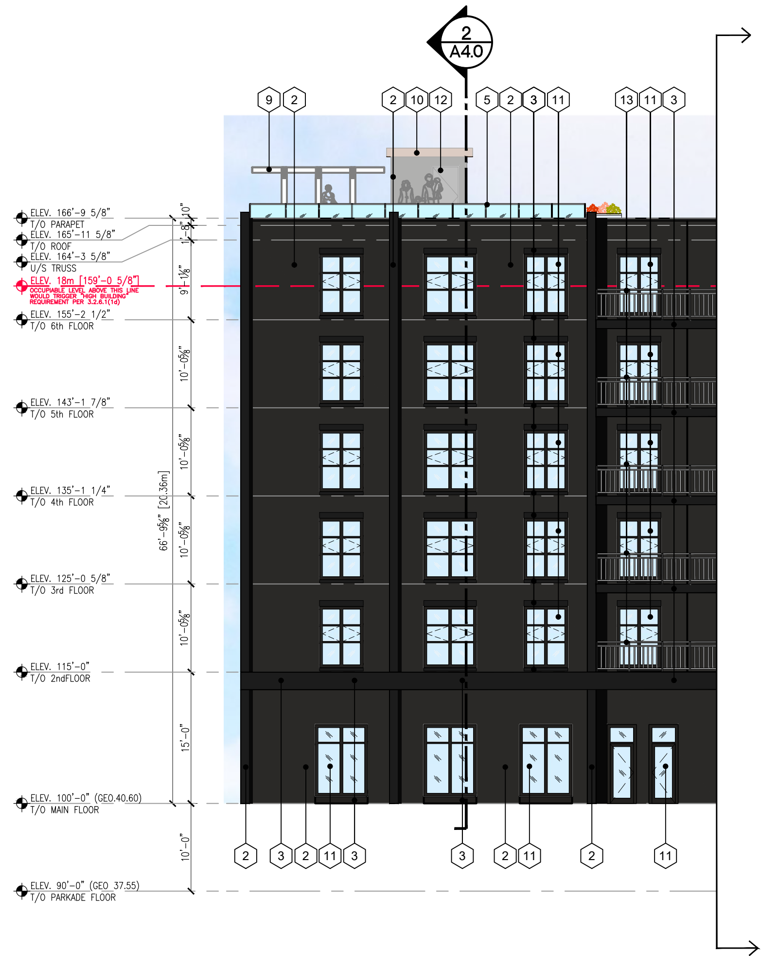
1 SOUTH-WEST ELEVATION A3.1 3/32" = 1'-0"
