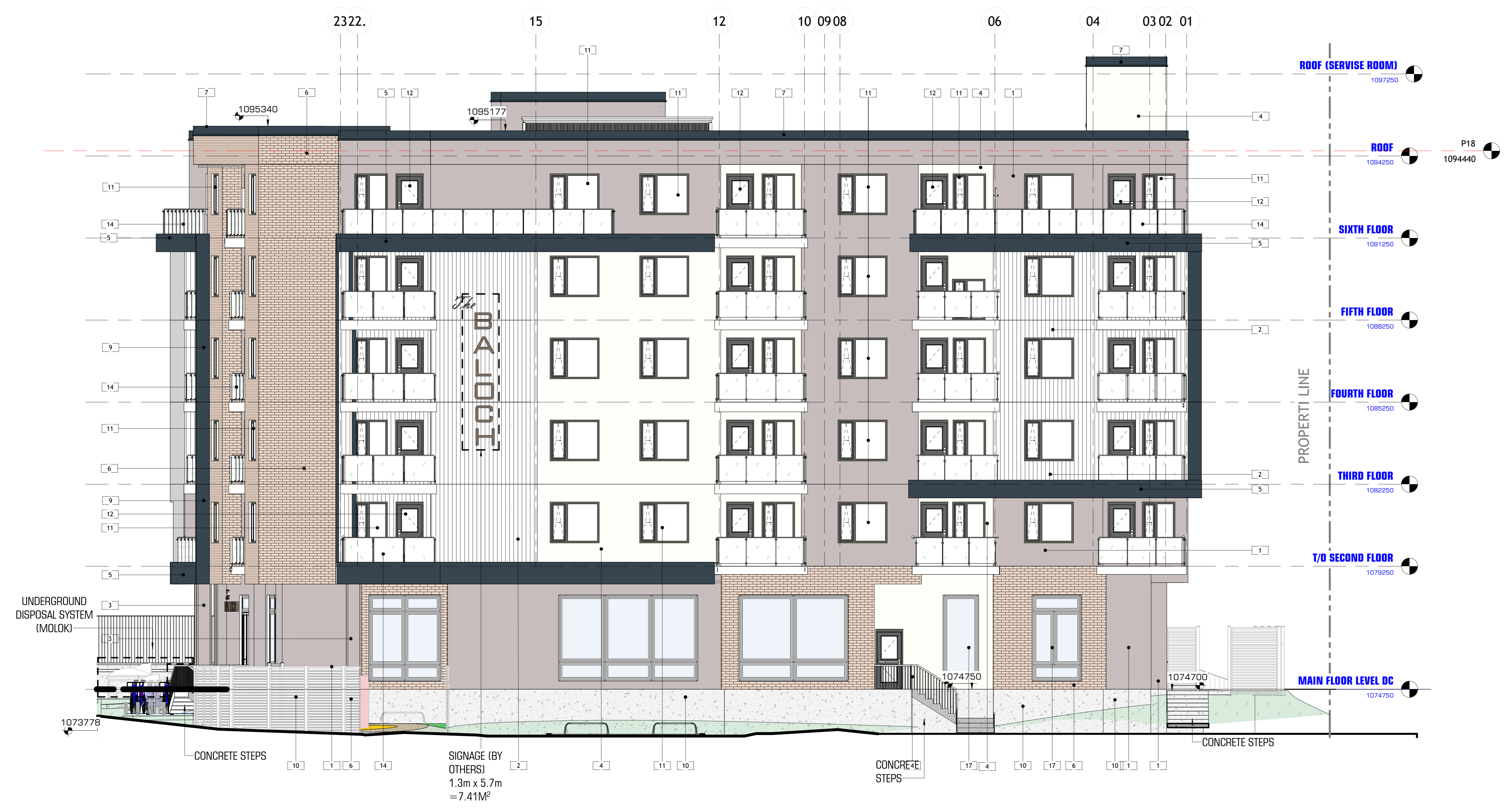
1 WEST ELEVATION - VIEW FROM EDMONTON TRAIL 1 : 75
