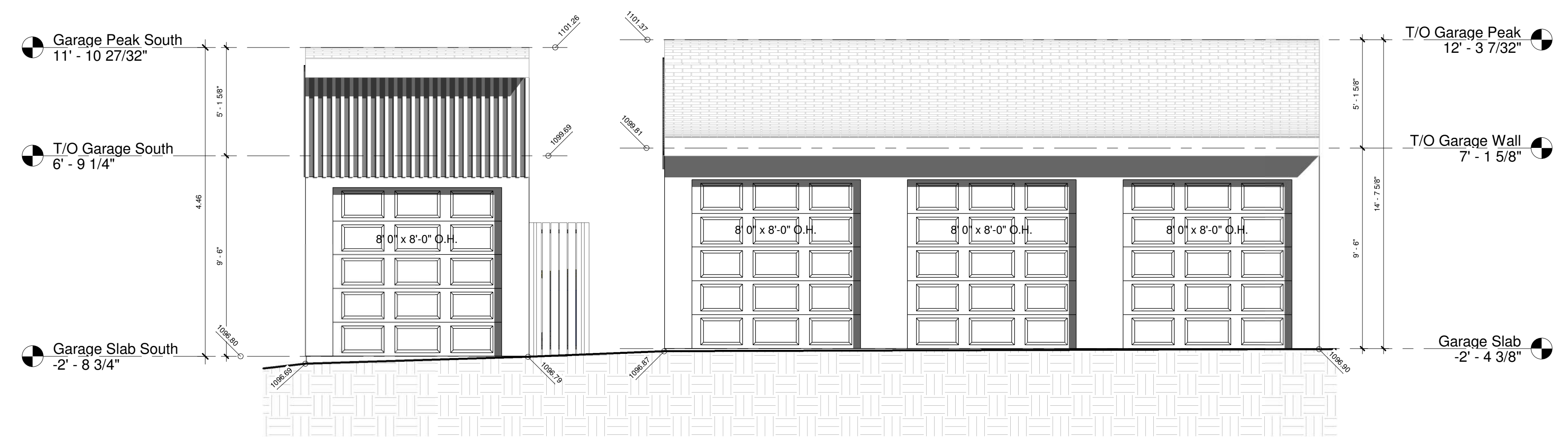
① Garage East Elevation 1/4" = 1'-0"
