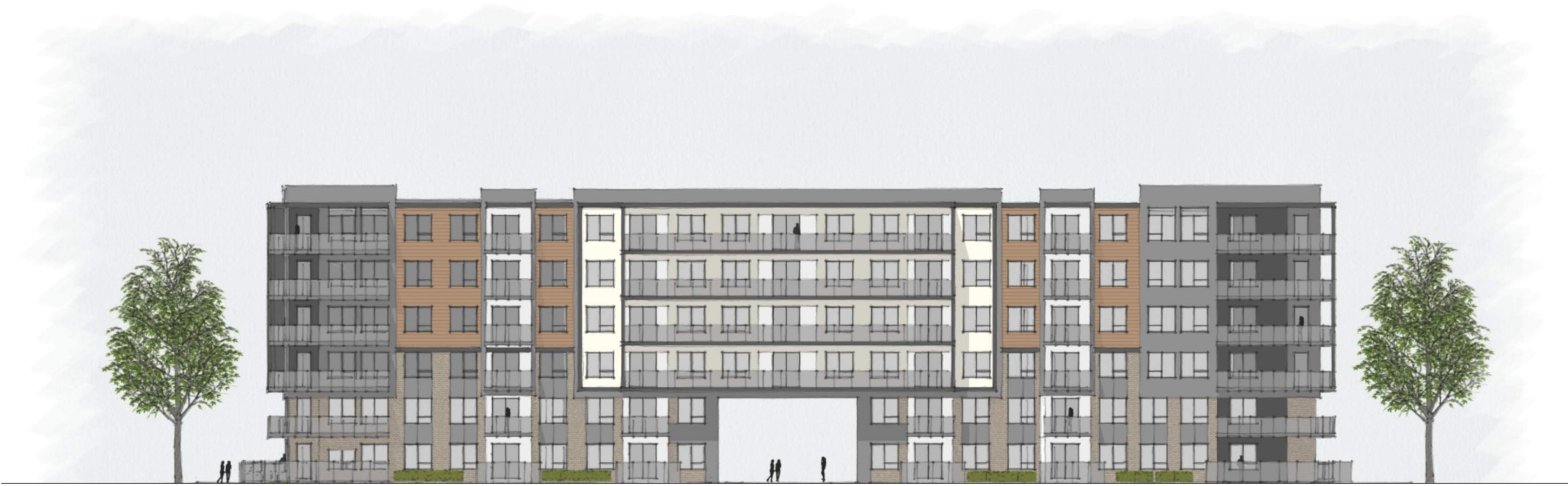
SOUTH ELEVATION WITH BREEZEWAY
